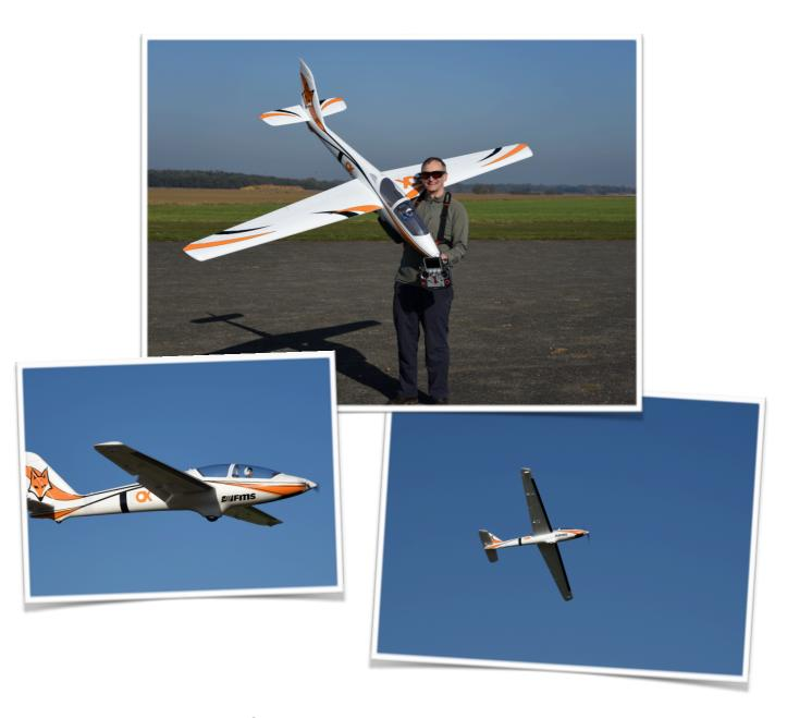
This is the FMS Fox 3m foamy, electric powered with 6s 4000 battery. Flies beautifully, but heck its a lump to hold in a moderate breeze.
