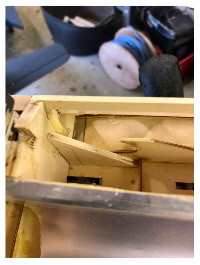
That completes the strengthening work around the U/C so it's onto the fitting of the longerons and balsa sheeting.
