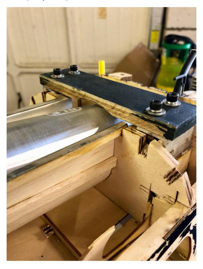
Next up, a couple of strengthening formers for the U/C which also provide some support for the firewall:
