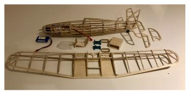
I took a punt on finished weight and have overpowered it possibly with a 10g brushless motor and 2S battery. On the other hand the finished all up weight of 77g compares very well with a similar sized eFlite UMX SBach. Yet to fly, yet to find out! Incidentally, finished for free flight the auw is likely sub 30g.
