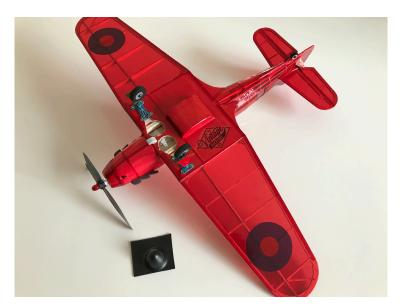
The model is covered with Solite transparent red instead of the very nice tissue supplied, with the paper/covering process extended to behind the cockpit to imitate the standard Hurricane metal sheeting look. Insignia were downloaded from The Vintage Model Company and printed onto decal paper from MrDecalPaper.
