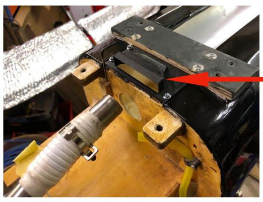
And fitted to force cooling air down through the can tunnel.
