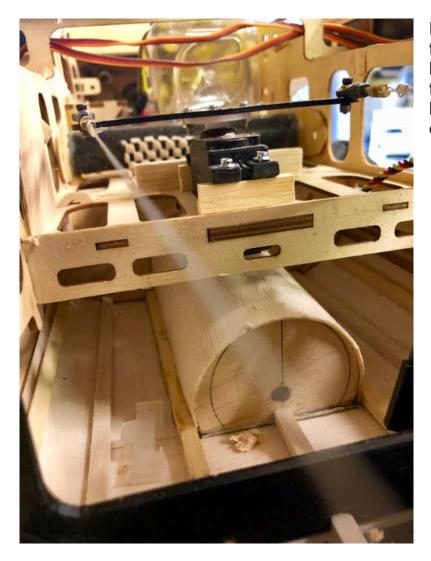
Having spent far too long on this part I decided to rest my brain and tidy up a couple of things inside the fuse. Firstly I had to raise the rudder servo due to the new can tunnel.
