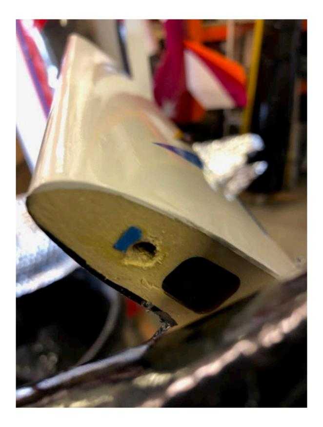
But how to fit a new dowel if I can't pull the tail away from the fuse? answer was to make a long dowel that went right through the fuse and would also serve for the other tail half.
