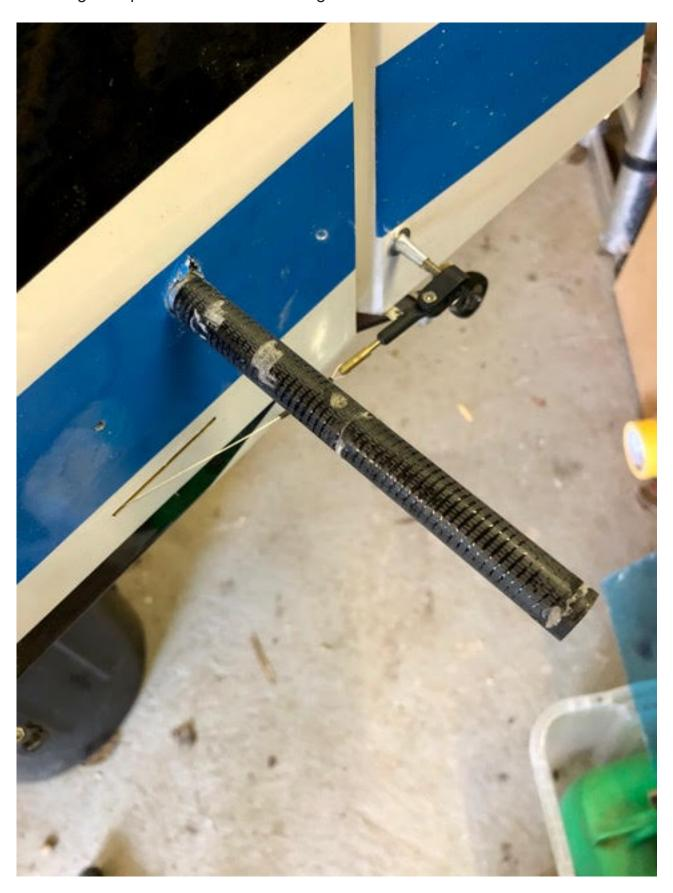
At least I was now able to bend the alloy tube straight so that the broken half sat parallel to the fuse, but in doing so the dowel locator pegs had to be cut off. This meant that I then had to somehow fit new ones but I couldn't get the tailplane off to drill out the old one! Using a small drill bit at an angle I managed to remove enough of the dowel.
