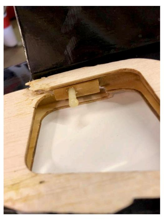
The wing tube pulled out from the wrong half!
