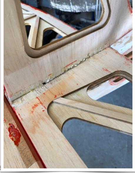
Some of the previous repairs (U/C ripped out!) needed the hot air gun (which I was now using to remove the covering)
