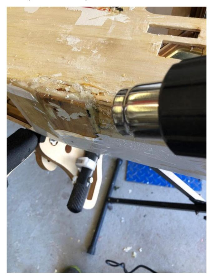
And a bit of a gooey mess left in places which needed the help of a scraper to remove.
