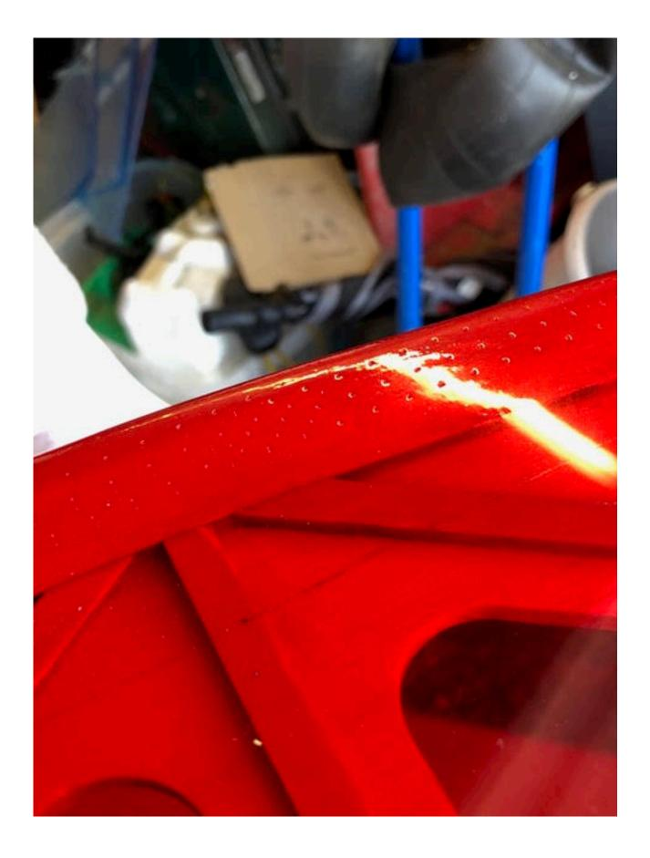
Another tip I remembered was to iron on a strip of film at the junction of surfaces such as tailplane to fuse, this makes the final covering joint less critical!
