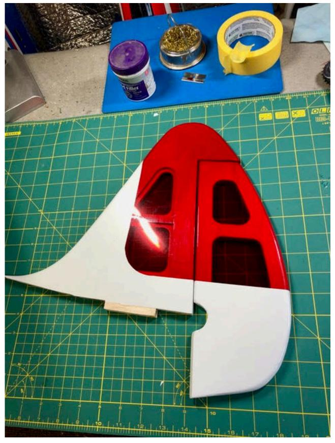
To assist the shrinking I remember a tip I was given a long time ago, drill some air holes to allow hot air out when shrinking film
