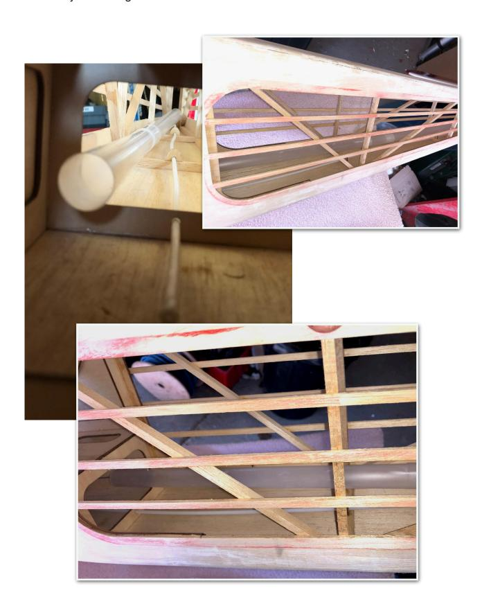
With that now sorted I turned my attention to the battery hatch using new formers created on the 3D printer
