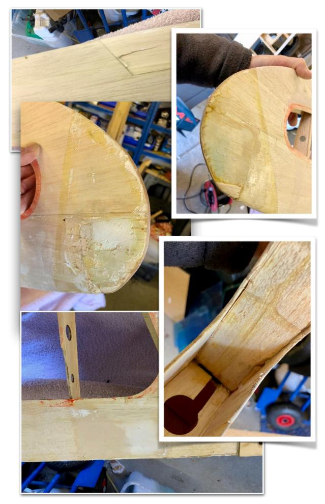
Having removed the covering I then set about cutting out the repair balsa mainly so that I could see 'underneath the skin' to see the exact extent of the damage and the repairs. I ended up with this.
