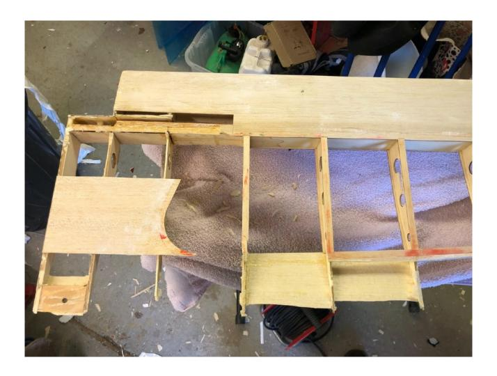
As I have to carry out fairly extensive repairs in this area I have decided to convert the wings to have flaps. Later Rascals are now supplied with flaps so it's more of an upgrade really! I now need to order some more balsa from SLEC as I haven't got any of the correct thickness of the correct grade (hard).
