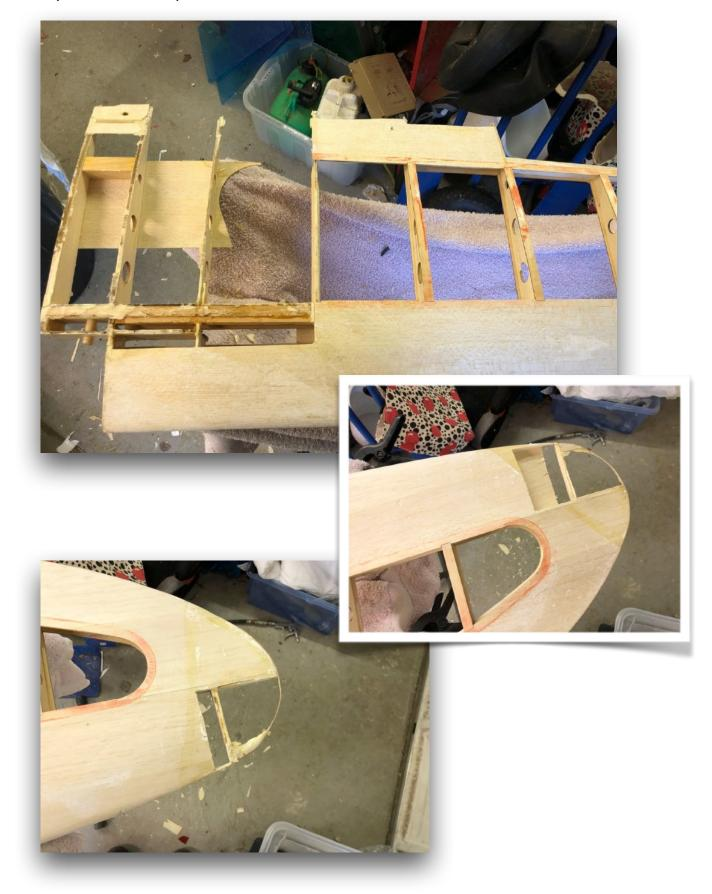
You can see that the TE section, inboard of the aileron has mostly been cut away.
