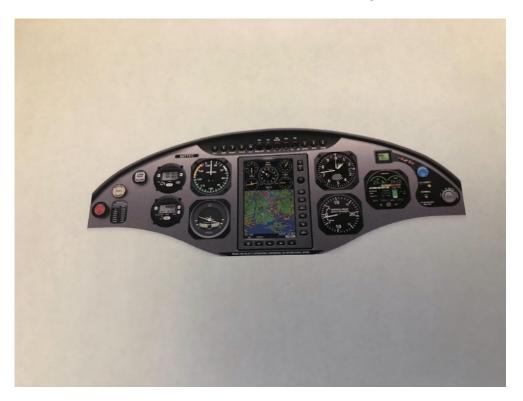
In my 3D print software, Fusion 360, I designed a dash with cut outs for some of the instruments
