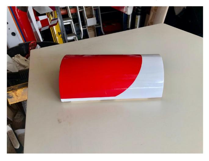
And yes, there is a slight crease in the covering and you may ask why doesn't it go down to the bottom edge. The reason for this is that I don't like an edge of film right on a small edge of structure as it can lift. Well that's the official reason but the truth is I cut it too short!
