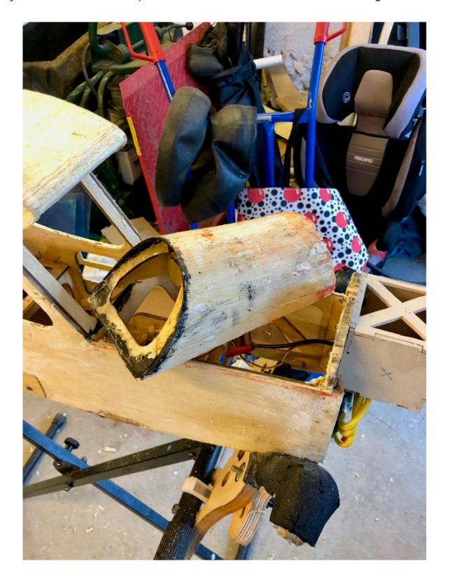
But I wasn't too happy with either the condition of the existing or the shape of the rear of it as a 'real' dashboard certainly wouldn't be sloping back the way this one is, and yes I know this isn't a scale model but I want it to look a little bit more scale! So I remade the hatch using a combination of 3D printed formers and balsa.
