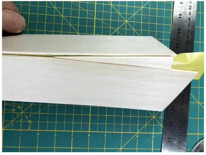
Once dry I then wet the outside of the sheet and bent it over the formers and left it to dry. This gives it the basic curved shape and makes sticking it onto the framework easier.
