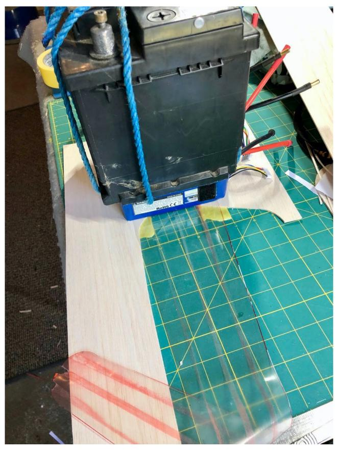
These have also been left to dry overnight but I had one last job I wanted to get done today and that was to cut out the new flap servo mounting plates using the good wing as the template.
