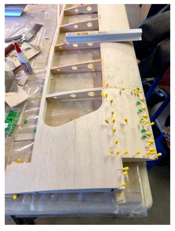
Followed by the second and third. And whilst that is drying I cut out the sheet for the underside of the wing.
