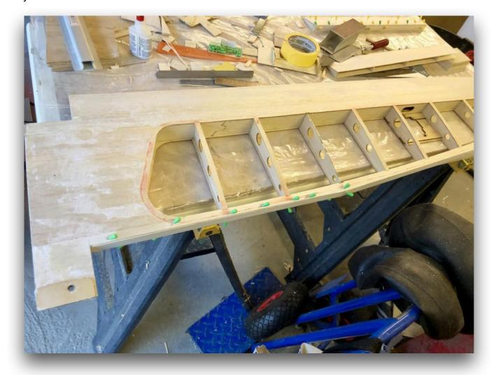
The new flap with its top sheeting added and the wing cut off ready to be converted into a flap.
