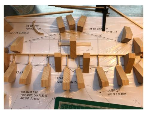
Gluing it all together almost defeated my steel and magnetic building board. There just isn't room between the parts to retain the spars; prop all of the edges; fit each rib centrally on the spar and leading/training edges.
