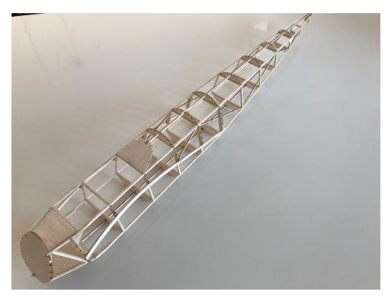
And finally with all bar two side formers fitted, top and bottom keels are in place (straightening the awry lower rear formers in the process), plus gussets added to brace the rear of the wing saddle.
