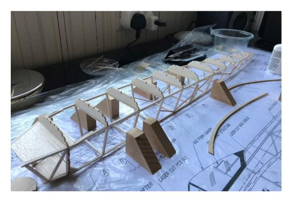
And immediately fell into the trap of too little time spent concentrating on the build in hand. I contrived to place them all square to the sticks forming the base of the inner trapezium shape, overlooking the rise towards the tail, leaving the rear formers all slightly angled backwards.
