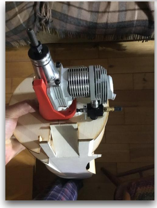
This was the problem I encountered trying to sort out the best positioning for the Laser. As you can see, the carb sits right up against the bulkhead.
