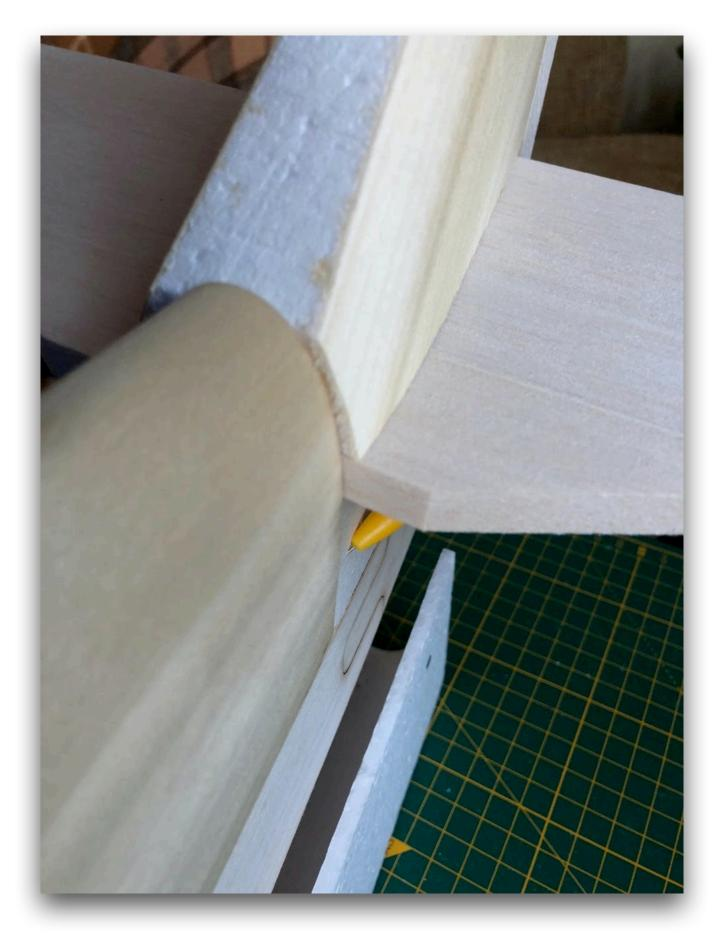
So I left that until later and concentrated on getting the fuel tank mount sorted, bearing in mind that a Laser needs the fuel tank to be at, or lower than the carb. I also fitted the servos into their final positions.
