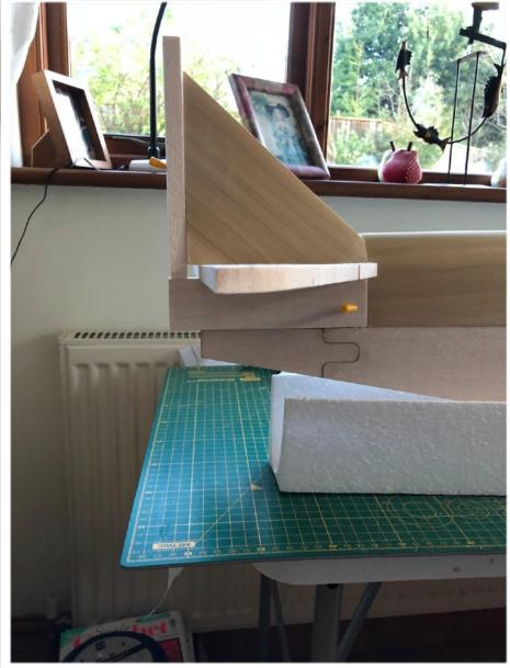
Fortunately the fin is also veneered foam with a balsa LE and rear post but work will be needed to fair the fin into the fuse.
