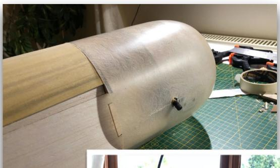
The turtle deck was fitted which makes short work of that curved section of the fuse so I now started to look at the tailplane and fin assembly.
