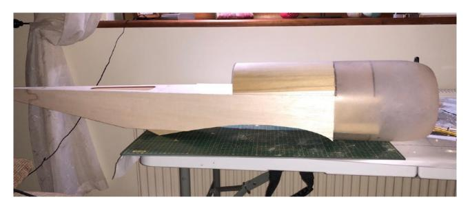
This is the bulkhead and tank bay but you can also see the piece of fuse angled in, that is for the airflow to the carb.
