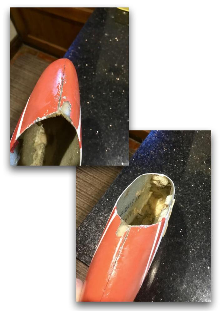
Rubbed down and ready for glass fibre strengthening / joining.
