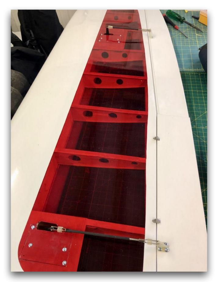
Then it was back to the tail end and I fitted the fin, making sure that it was upright (unlike before the refurb!), and elevators all using flat cyano hinges from SLEC. I had already decided to do away with the rudder pull / pull system and have a rear mounted servo like the one for the elevators.
