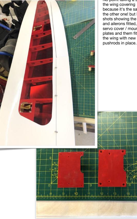
No point taking a shot of the wing covering because it's the same as the other one! but here are shots showing the flaps and ailerons fitted, the servo cover / mounting plates and them fitted to the wing with new
