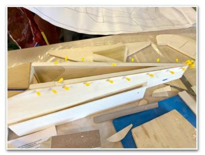
Whilst that was drying I dug out the tail pieces and remembered that 2 years ago I had the bright idea of a few changes to make it more scale like. One of these being hidden hinges and I had started the work on these on the fin / rudder. No getting away with not doing that on elevator then, so I stripped some sheet balsa down to provide extensions to the tailplane TE which could then be sanded down to form the recess for the elevator LE.
