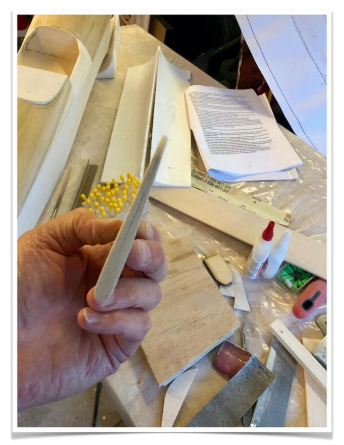
Going back to the strip balsa I used for the TE, I already had a large SLEC balsa stripper but I needed something a little bit smaller. So over to the 3D printer and this was produced. It works really well. Not my design but available on Thingiverse.
