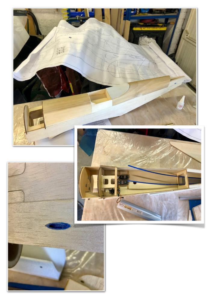
Then it was time to close in the bottom of the fuse with 1/8th balsa having first fixed  $\frac{1}{2}$  triangular stock to support it. The keen eyes will note a join in the triangular supports, the kit came with a length for each side but rather than having a small off-cut laying around I used it!
