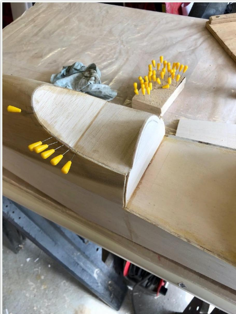
I then wet and bent some thicker balsa to form the new sides to the cockpit which made it easier to glue in place. (I used the cowl as the former to bend the balsa around).
