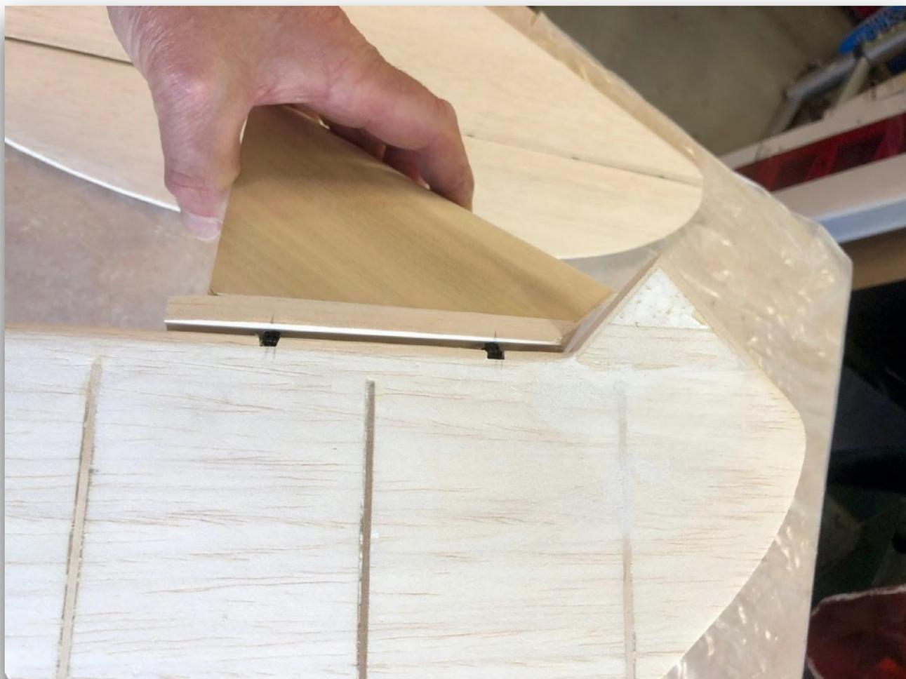
That's about as far as I wanted to get with the fuse so I moved onto the wings. The first job was to mark and cut out the recesses for the retracts and wheel wells. The retracts are mounted on a ply plate which has to be let into the wing at an angle. After removing the veneer I then cut out the foam using an old penknife which has a nice long blade and is very sharp!
