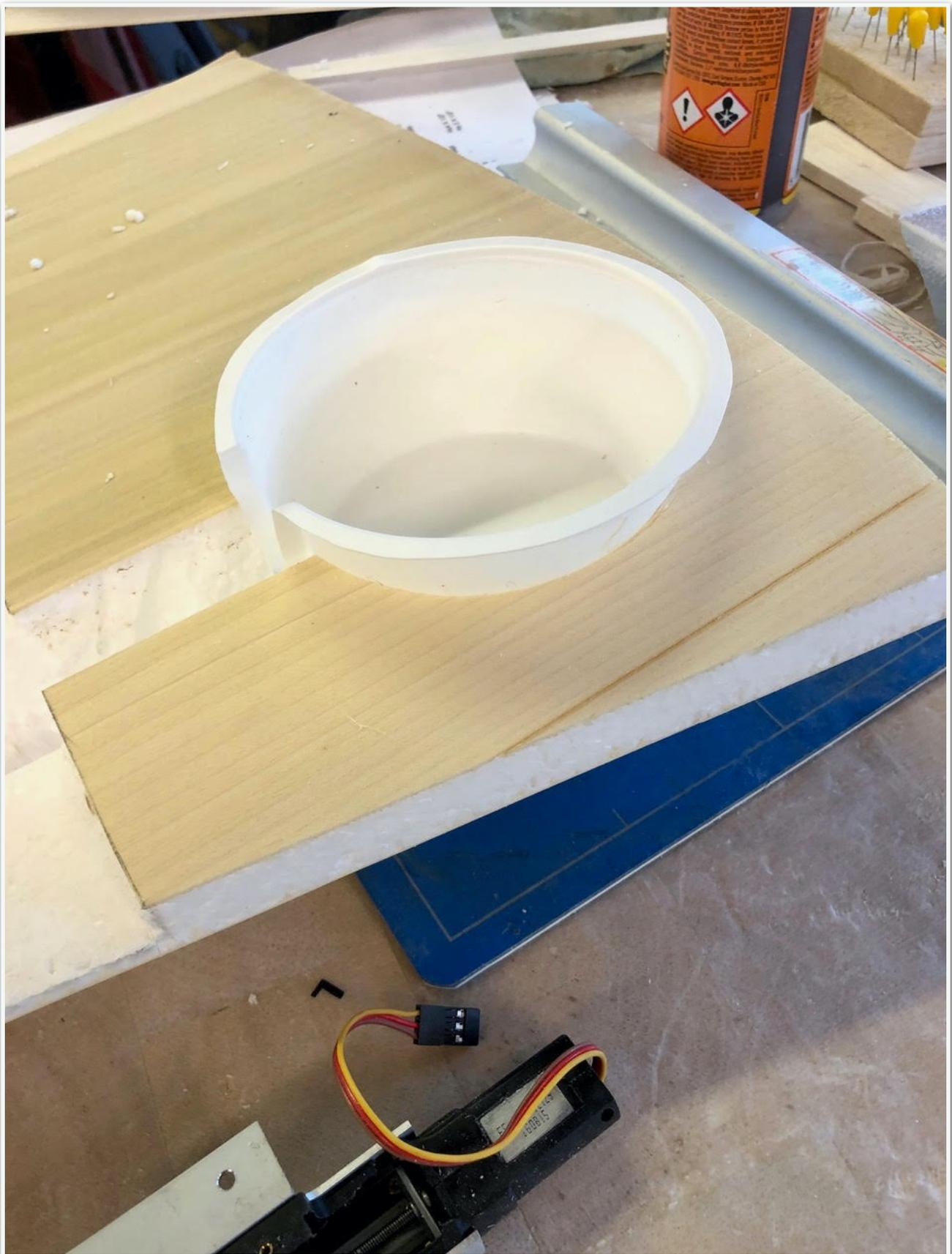
And the soldering iron was used again to cut out slots around the ply retract plates to facilitate the fitting of the balsa sides to the retract 'bay'
