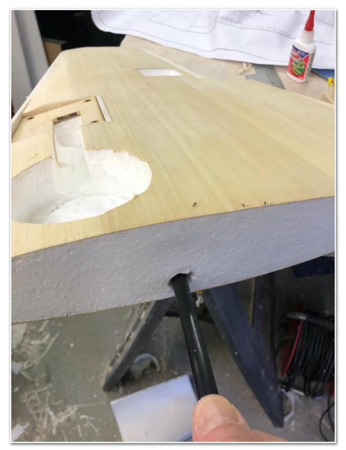
I also cut another channel at an angle to the one shown above exiting at the bottom of the wheel well. I want all of the cables to exit the top of the wing on one place as I will be using a Maxloc 4 way connector so that I only have one thing to plug in when I mount the wing on the fuse. More by luck I managed to get the channel to exit right at the back of the servo pocket.
