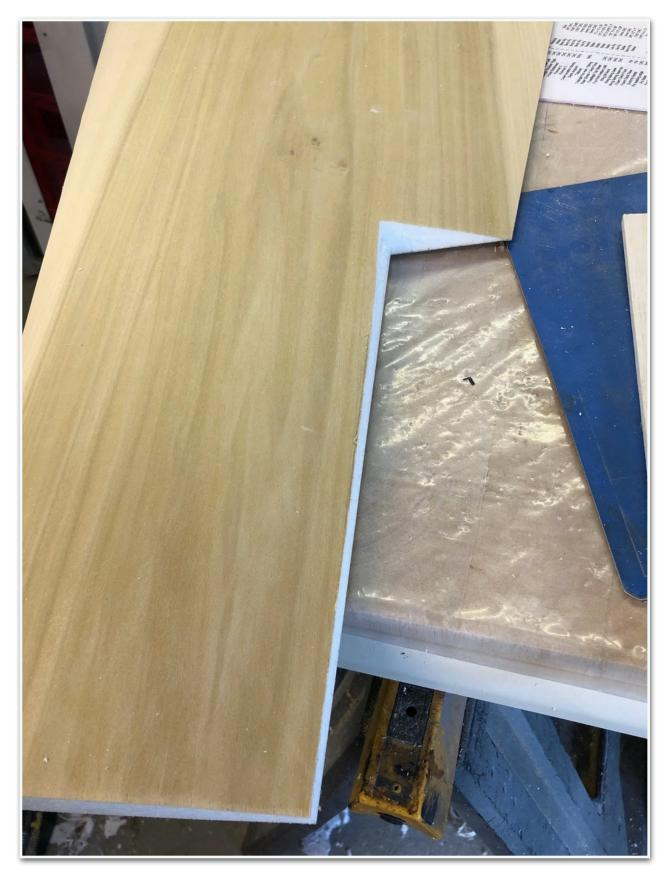
The ailerons were cut out using a wide bladed razor saw and then the edges were trimmed to receive the false TE.
