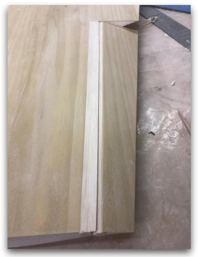
Having cut out the servo pockets (soldering iron foam cutter) I then decided to tackle the cable routes for the aileron servos and the retracts using a sharpened length of CF tube to core the channel out.
