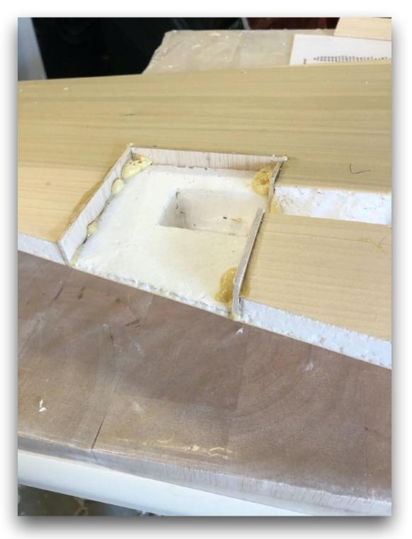
The plastic wheel wells were cut down to size and I will reuse the bottom off-cut inside the well.
