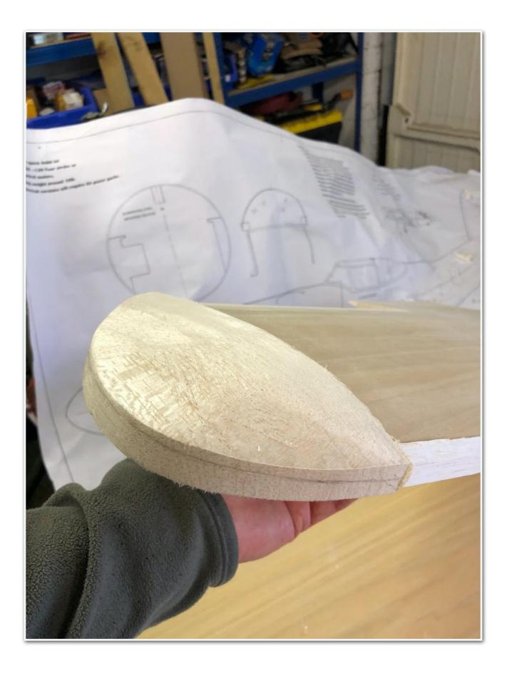
Hard points in ply were let into the ailerons, these will be the mounting blocks for the control horns.
