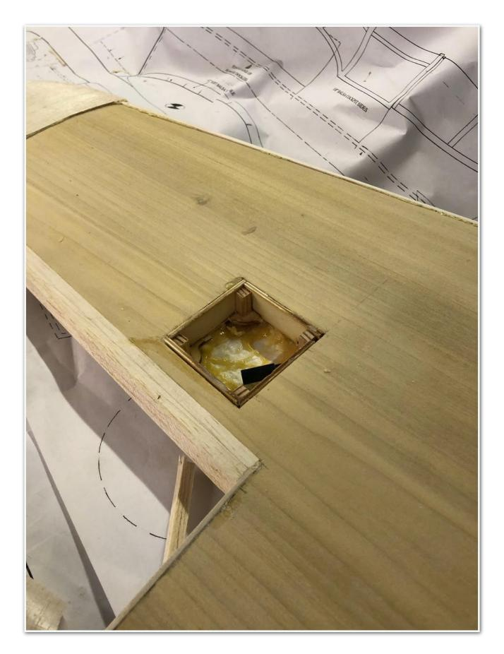
And I started to cut / carve the wig tips to shape. They were quite a big lump of balsa so I started with rough cuts using a hand saw, then used the razor plane followed by the Permagrit block
