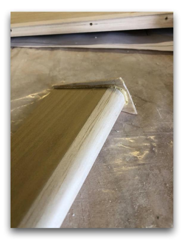
Now over to the concealed hinges and fitting the Robarts which was not that straightforward given the varying taper on the hinge line. I first cut a short length of barbecue skewer and sharpened one end to act as a marker. After marking the centre line, shallow holes were made in the wing using a rat tail Permagrit file and the marker inserted. I then pushed the aileron into position and the hole positions were transferred via the sharpened marker.
