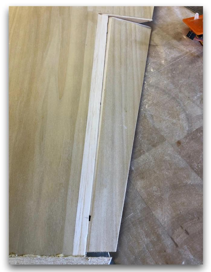
Just got the end plates to put on the outer ends of the ailerons, hence the gap.
