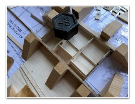
I added rib 1, then used it and loose fitted ribs 2 and 3 to get the spars in place, both forward and aft of the temporarily fitted brace.
