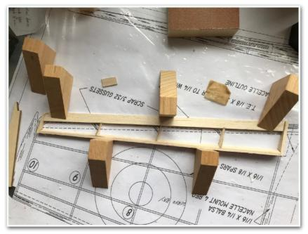
Along the way I also knocked up a couple of ailerons. I had drawn a 'plan', but to be fair 'bodged' would be an adequate description of the process.
