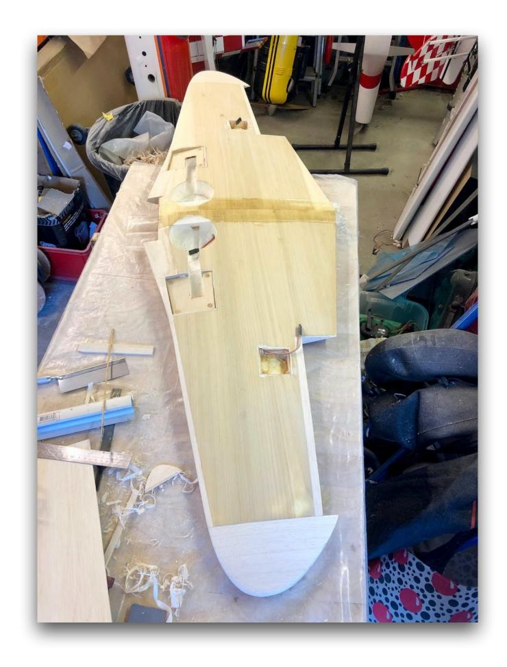
Whilst that first coat of epoxy was curing I continued with work to the tail pieces starting with the hard point for the rudder.
