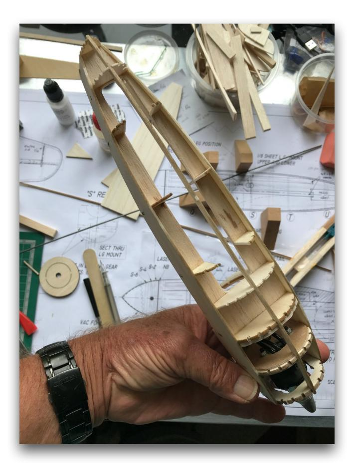
Next in line, fit the gear mechanism and ensure square and true, check nacelle fit and build the other one, fitting the gear servos in the the wings. A bit of reinforcement to forward spar and top sheet the wing.
