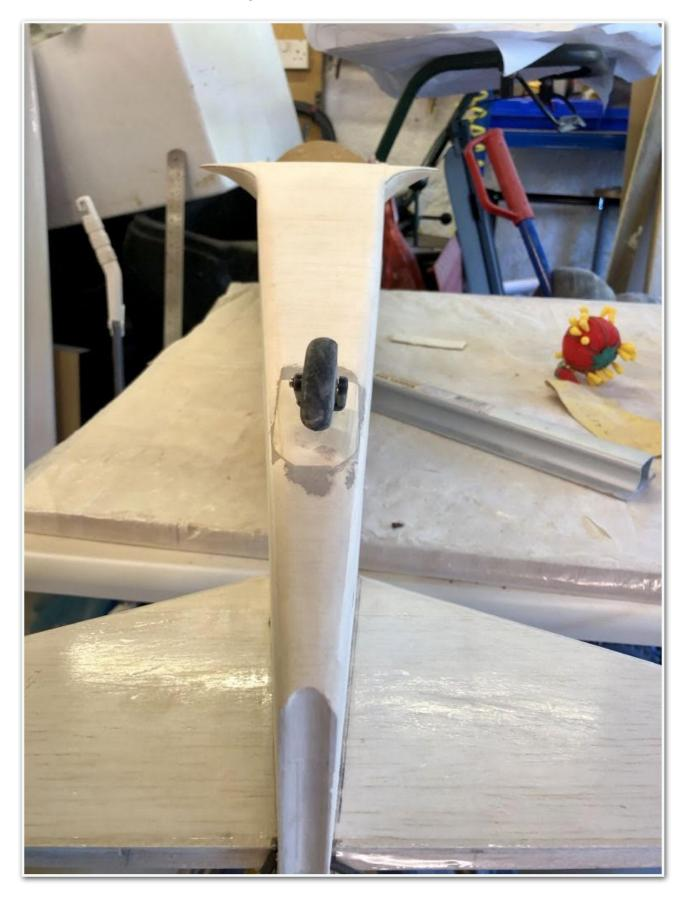
Whilst looking at photos of the full size I realised that there is a fillet between the fin and tailplane so I've stuck in some triangle strip which will be sanded to a concave profile.
