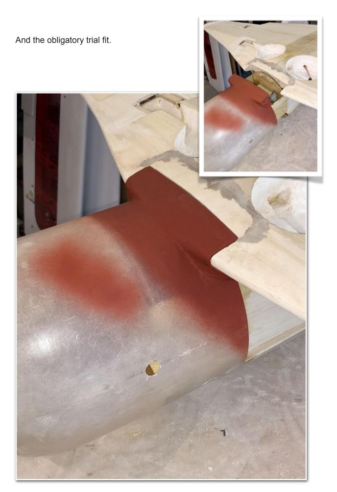
Eventually, the first piece of laminating film goes onto the wing. My roll of film is only 300mm wide so there has to be a join which will be feathered so hopefully won't be that obvious.
