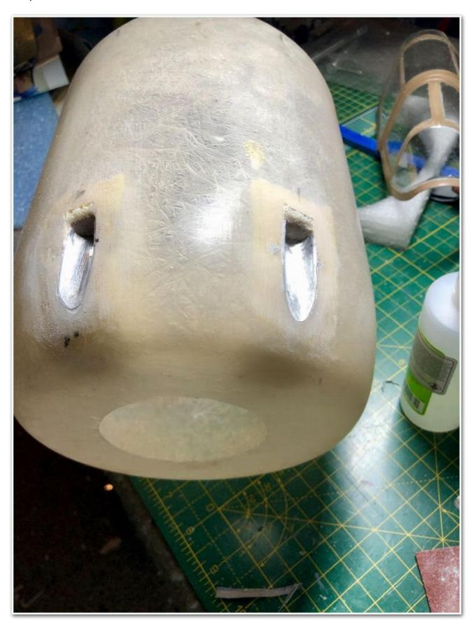
Finally I used aluminium tape to form the panel.
