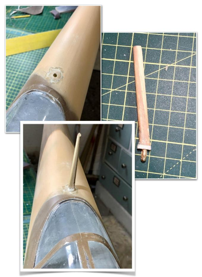
Then it was out with the yellow paint for the spinner and cowl ring, followed by the 2 aluminium (tape) cowl bands and the machine gun barrels made from some brass tubing.
