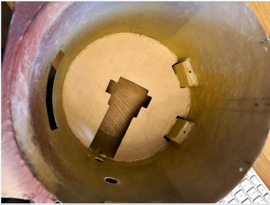
Engine (Laser) air baffle fitted (3D printed and laminated with ply)
