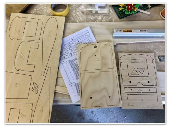
Quickly progressed to the formers which have to be removed from their parent sheets but you can see the quality of the CNC routed parts
