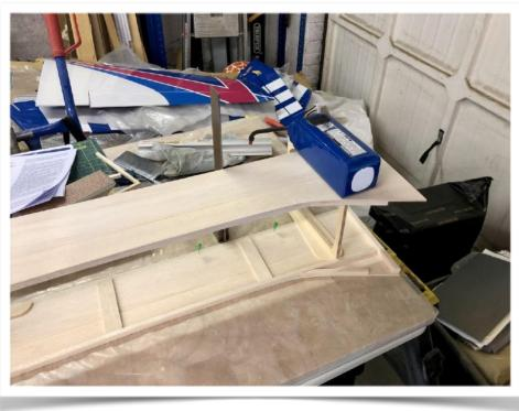
I keep meaning to make myself a jig but progressed without one using set squares and front to back aligning to make sure everything was square. To be fair having made sure that the front end was square when I fitted the first 2 formers, very little adjustment was necessary to make sure the fuse wasn't twisted when it came round to pulling in the tail end but a jig would have made it easier (make one!!!!).
