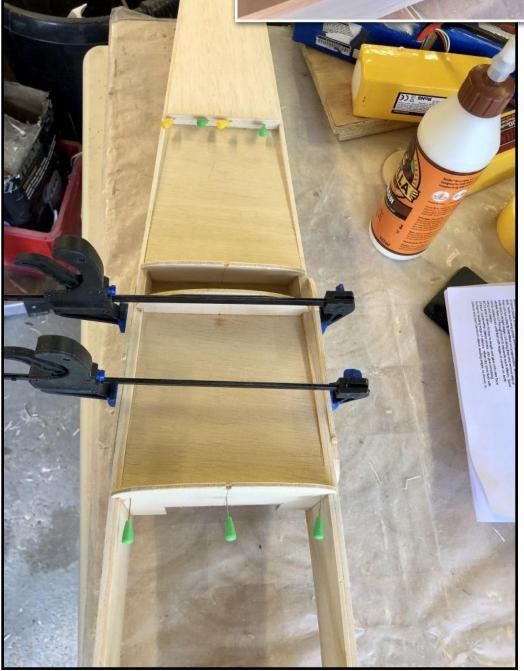
Cockpit floors added, I've gone for the '2 seater' option which gives a longer canopy which I think suits this model, so there are 2 floors to fit. Also fitted the balsa sheeting to the top rear of the fuse.
