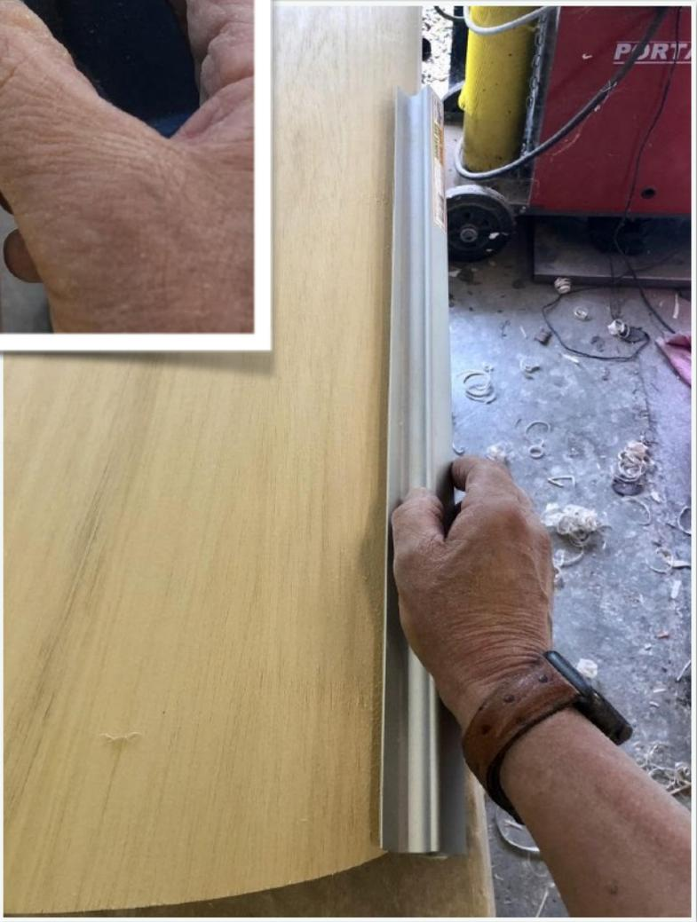
Wing tips added and sanded to blend in to the wing
