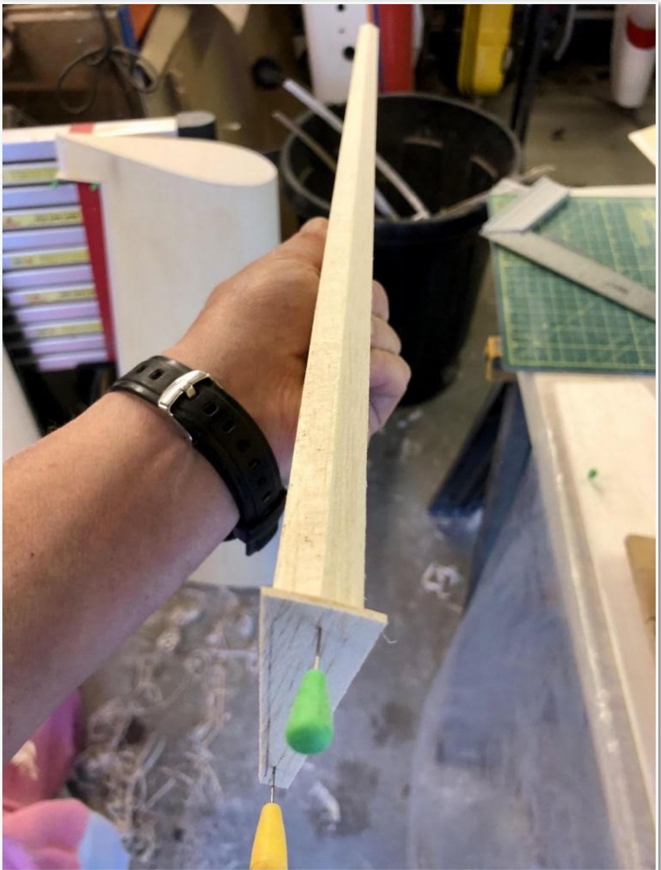
And the balsa end plates were also fitted to the ailerons (see photo above) and the wings.
