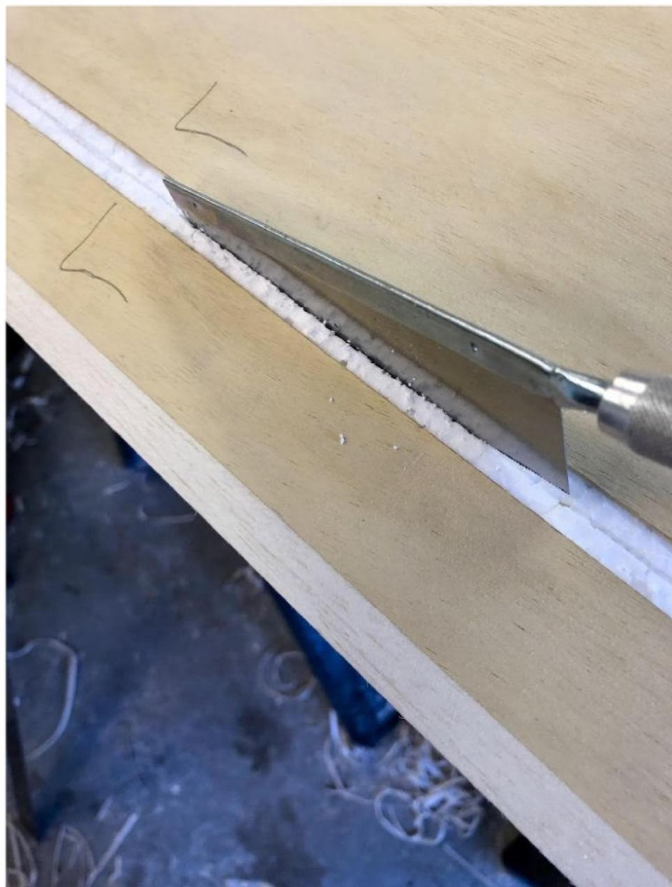
then the razor saw was used to cut through the foam.
