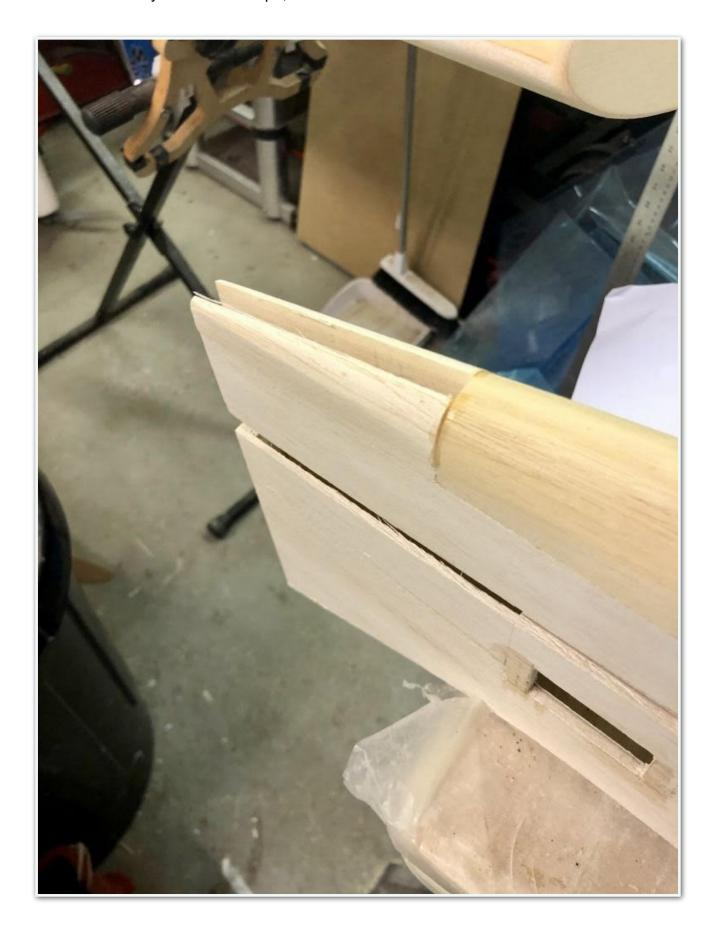
The instructions say to glue triangular hardwood pieces to the 3 sides between the wing LE and engine bulkhead, I decided to edge all 4 sides. The UC plate had the T nuts fitted and then was glued to the fuse using Gorilla Glue.
