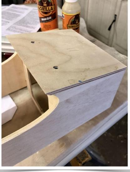
The supplied tail skid plate was undersized so I cut a new one from the ply sheet that the supplied one was in, not a real problem. I had thought about changing the tail skid for a wheel as I don't like the scraping sound on a tarmac / concrete runway but then thought of a novel idea for this, more later.
