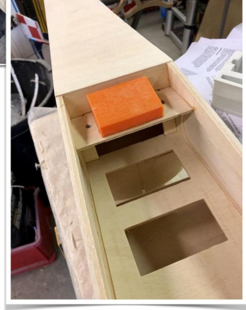
The instructions say to cut a slot out of the wing and then to glue the wing fixing bolt plate into it. I would rather spread the load with a ply plate sitting across the underside of the wing. And just checked to make sure it all fitted.
