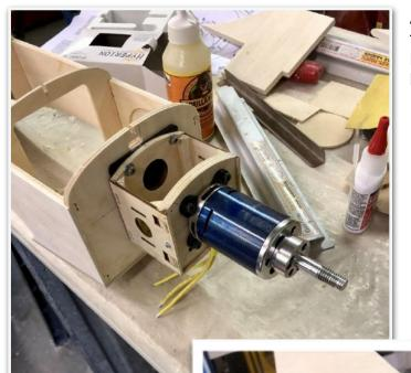
And a photo with the motor fitted. Yes, the threads at the end of the shaft are knackered, the joys of buying second hand, but they will be cut off.
