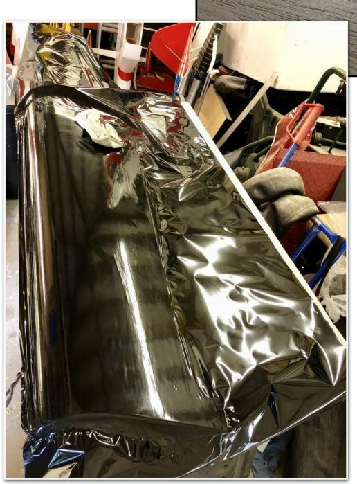
Notwithstanding this I started the covering with the underside of the wings, well actually I decided to do all of the black bits first, leaving the control surfaces until later as they will need the control horn hard points fitting first.
