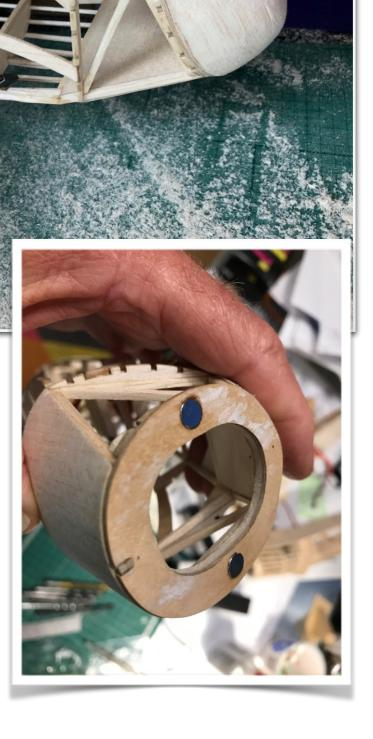
Added the forward top deck. I found the shaping of this really challenging and have ended with a compromise that looks about right, but is not as per the plan. This shot also shows the nose block after initial rough shaping.
