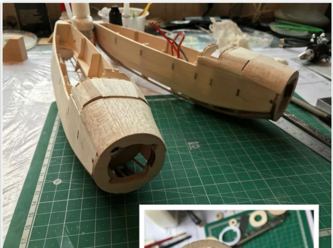
Through bad planning the prop drivers have ended slightly forward of the nacelle face. Happily this allowed for one of the 3/32" wheel discs be remodelled on each nacelle to bring the face neatly down to 45mm diameter as per the plan. Which is usefully a standard spinner size. Though not a 3 blade spinner that I can find.
