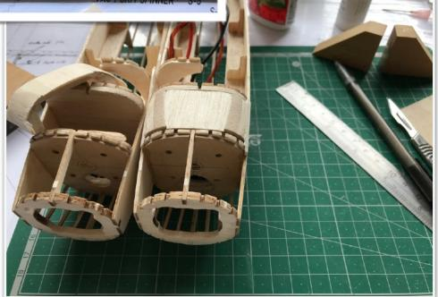
Permanently sheeted the first nacelle bay so that the whole top of the nacelles will ultimately be sheeted. Also, far too late, I increased the hole size for the motor power wires deep inside. Just too tight. Upper sheeting over the hatch to blend into the wing must wait until the nacelles are fitted.
