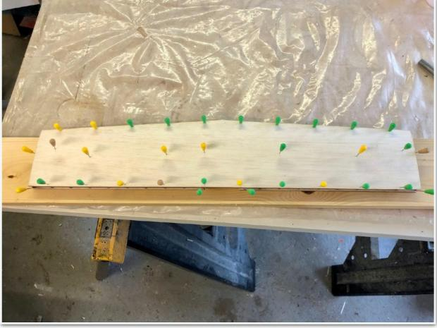
The fin assembly follows a similar pattern to the tailplane, a skeleton core with balsa outer skins. The dark brown pieces are ply doublers which add strength where the fin attaches to the tailplane.
