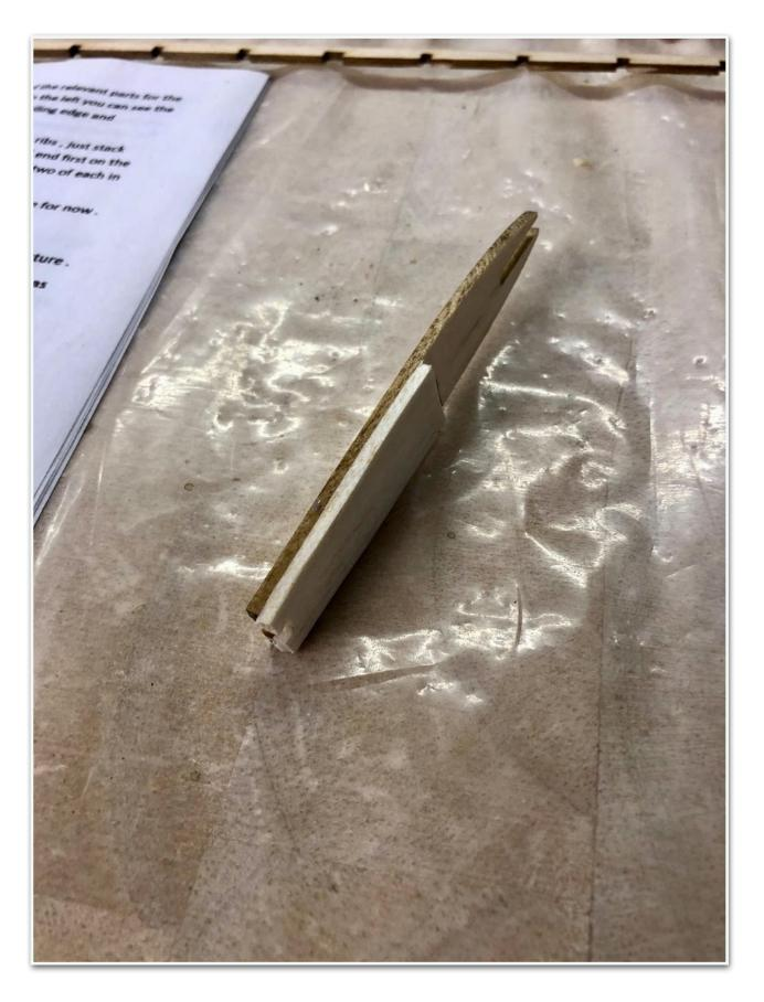
Just like a jigsaw puzzle the tailplane parts are slotted together and then the joints glued, the whole lot being a self jigging assembly. Balsa sheeting is then added to both top and bottom surfaces. Note the cut out in the top sheeting for the servo access panel.
