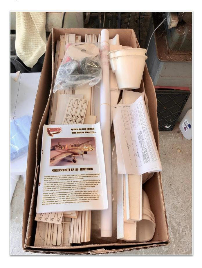
In typical Warbird Replicas fashion it comprises balsa built up fuse and tail and veneered foam wings and turtle deck with moulded plastic nacelles and cockpit floor. The standard of laser cutting is excellent with very little effort needed to separate the parts and very little excess burning of the balsa / ply.
