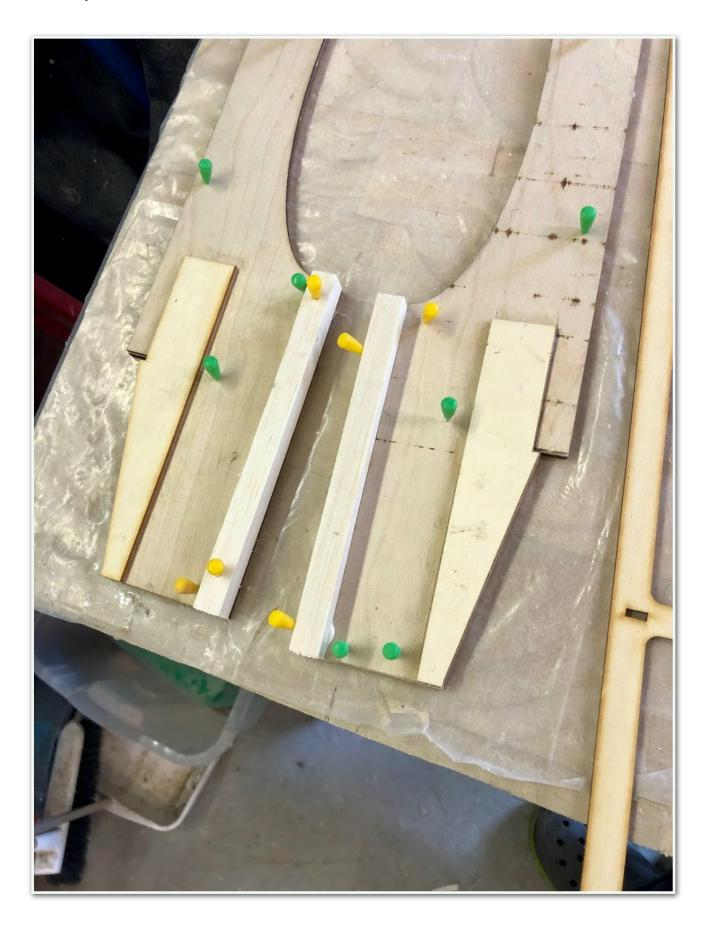
The fuse sides get glued to the crutch in the centre section only, I'll draw the nose and tail together after this section has dried.
