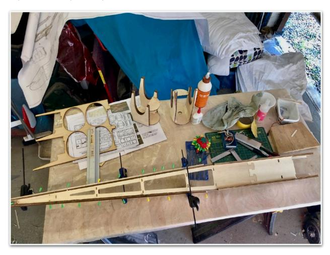
Before going any further I thought it best to fit the servo which will operate the rudders. I've deviated from the kit here as that calls for a bell crank assembly to be installed in the tailplane but I wanted to mount a lightweight servo as there will be less slop in the linkage and, as it turns out it will actually be lighter than the bell crank and pushrod! The servo is a Bluebird 7.5g one with 3Kg of torque (I use these on my F3K and F5J gliders).
