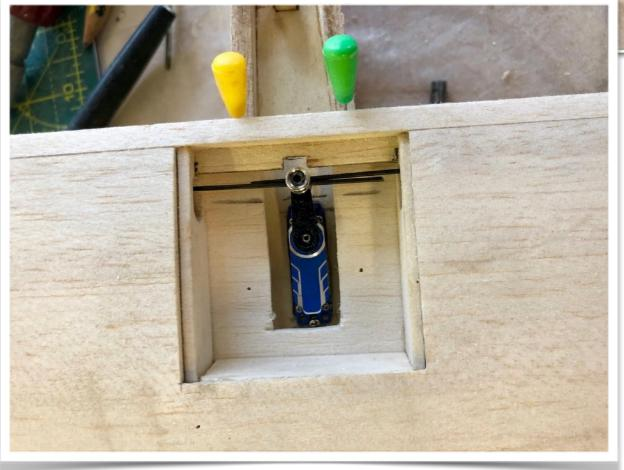
Once happy that this would indeed work, I set about covering the tail using laminating film for the fins and tailplane and Solartex for etc rudders and elevators. I then silver soldered a control horn to the elevator joining wire and was then able to glue the hinges in place.
