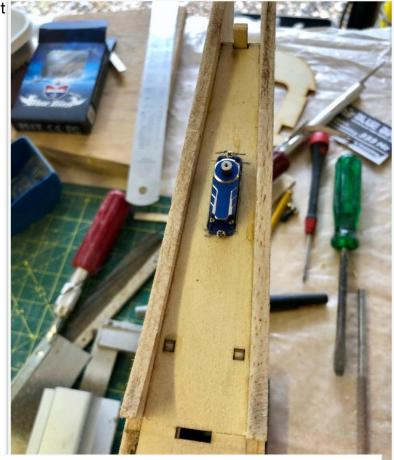
Just to make sure it will work I dry assembled the tailplane onto the fuse.
