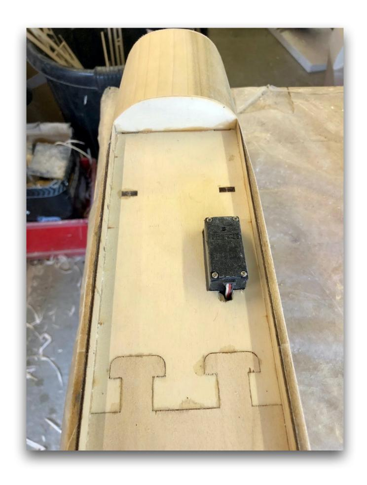
Now I could get on with fixing the veneered foam decks followed by lots of sanding to form the curved fuse.
