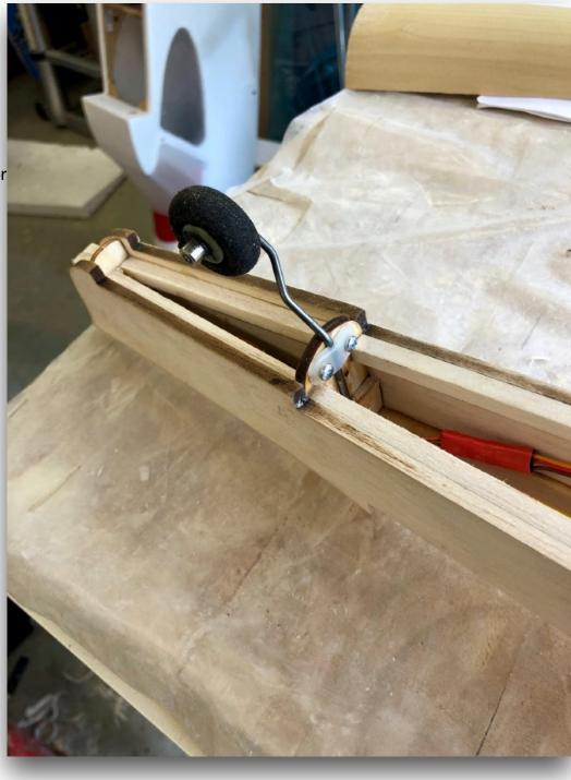
Next I fitted the extended servo cable for the rudder servo and a lightweight snake for the elevator.
