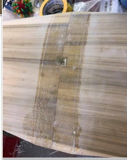
Next I marked out for the ailerons and flaps and removed a strip of veneer on the top and bottom of the wing.
