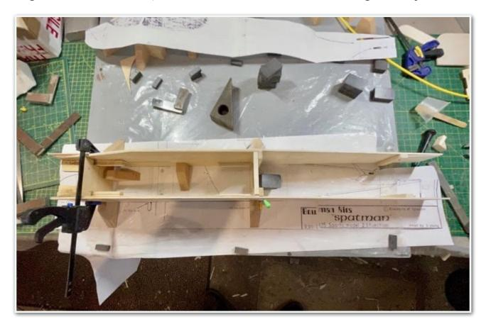
Servo tray and tank / throttle servo platform added.
