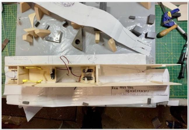
Some black spray applied to engine bay and fuselage sides brought together.
