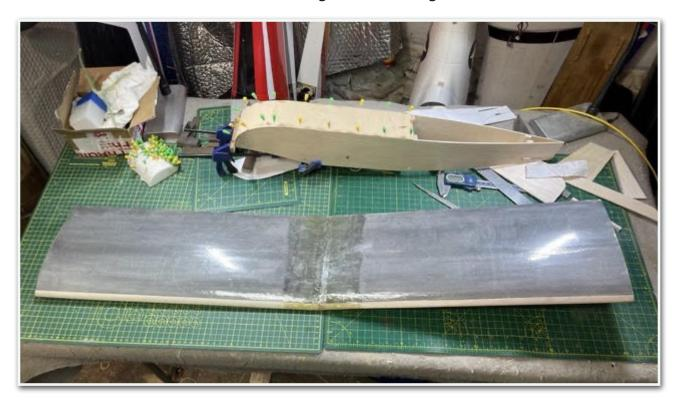
Control snakes installed and the balsa sheeting added to the fuselage, together with tail skid; I did think about fitting a tailwheel but decided to keep it as per the original (plan that is as mine never had U/C as I only flew from rough fields).
