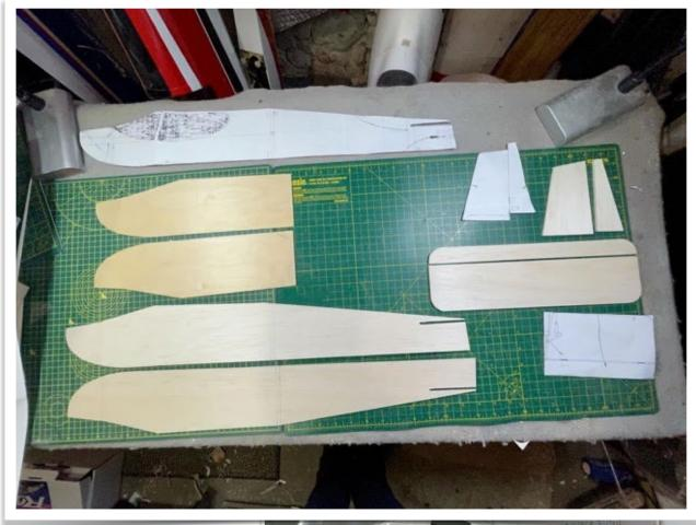
Made up the balsa former using my magnetic building board for the first time in ages
