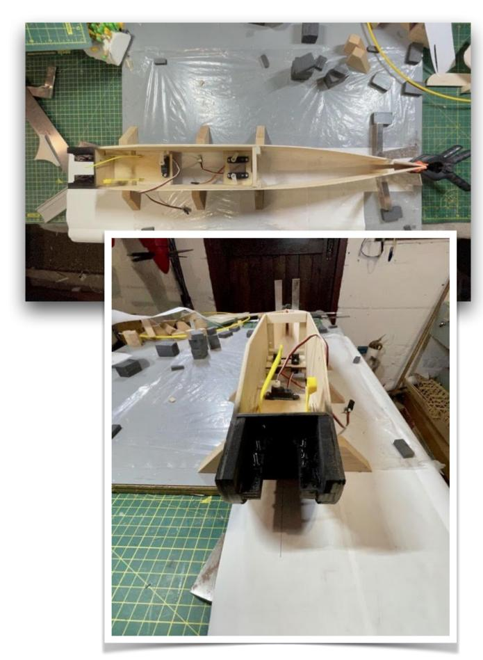
Underside ply sheeting was preformed whilst damp then attached. I've added a ply U/C mounting plate to the inside of the ply sheeting.
