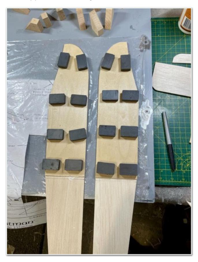
Engine bearers installed, front & mid former fitted and fuselage sides joined.
