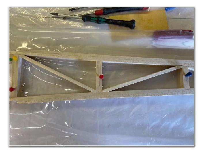
Then onto the front fuselage sides.
