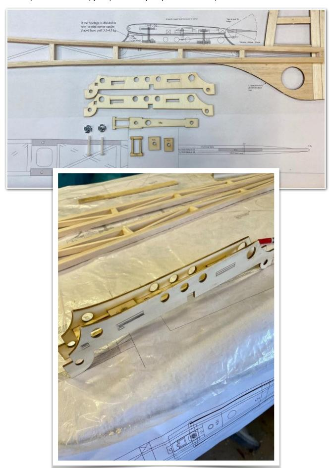
Whilst those parts were drying I got on with the fuselage cross braces but in doing so made a mistake. On the plan it refers to 5mm x 10mm which I took to mean that was for the cross bracing but looking closer at Dane-RCs photos they should have been 5mm x 5mm, no wonder I ran out of the 5mm x 10mm when I started the front fuselage!
