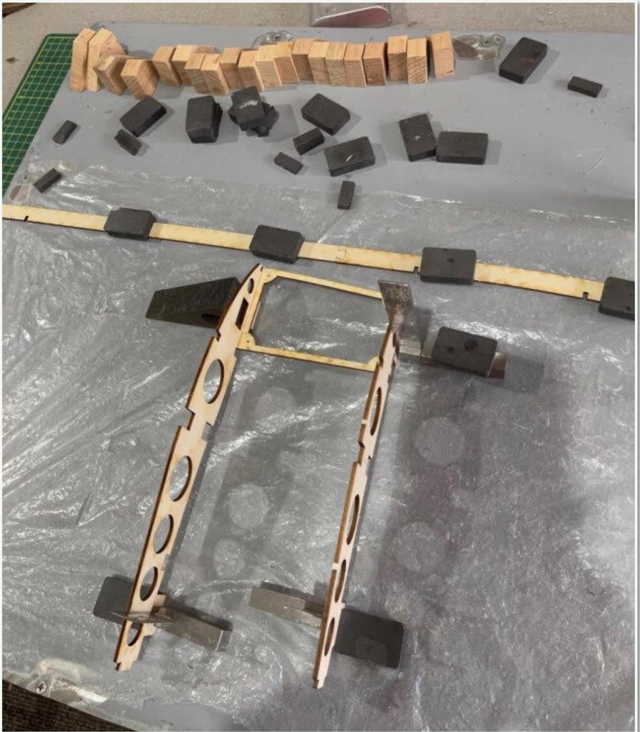
The wing joining boxes made from laser cut ply, nice fitting but I nearly clamped one too tight which would have prevented the ply joining tongue from fitting. 6 boxes in total.
