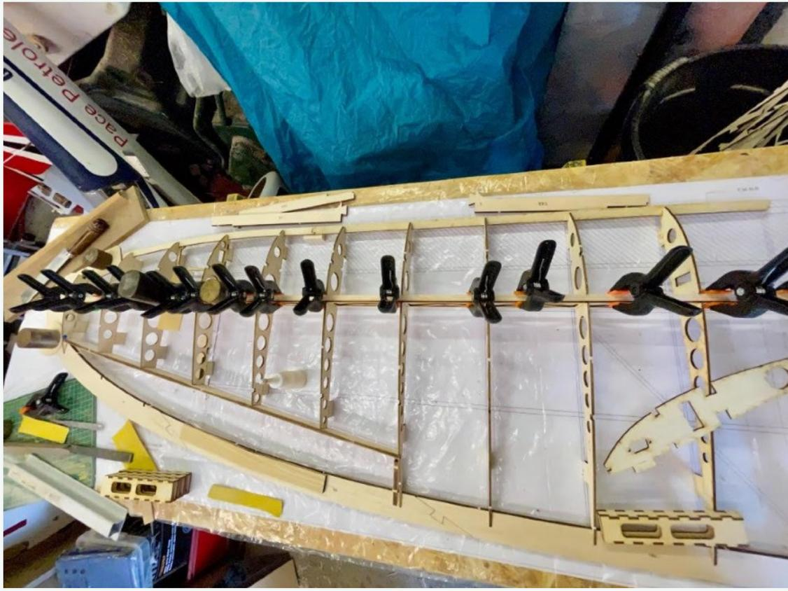
Front and rear spars added plus aileron riblets and box for wing brace.
