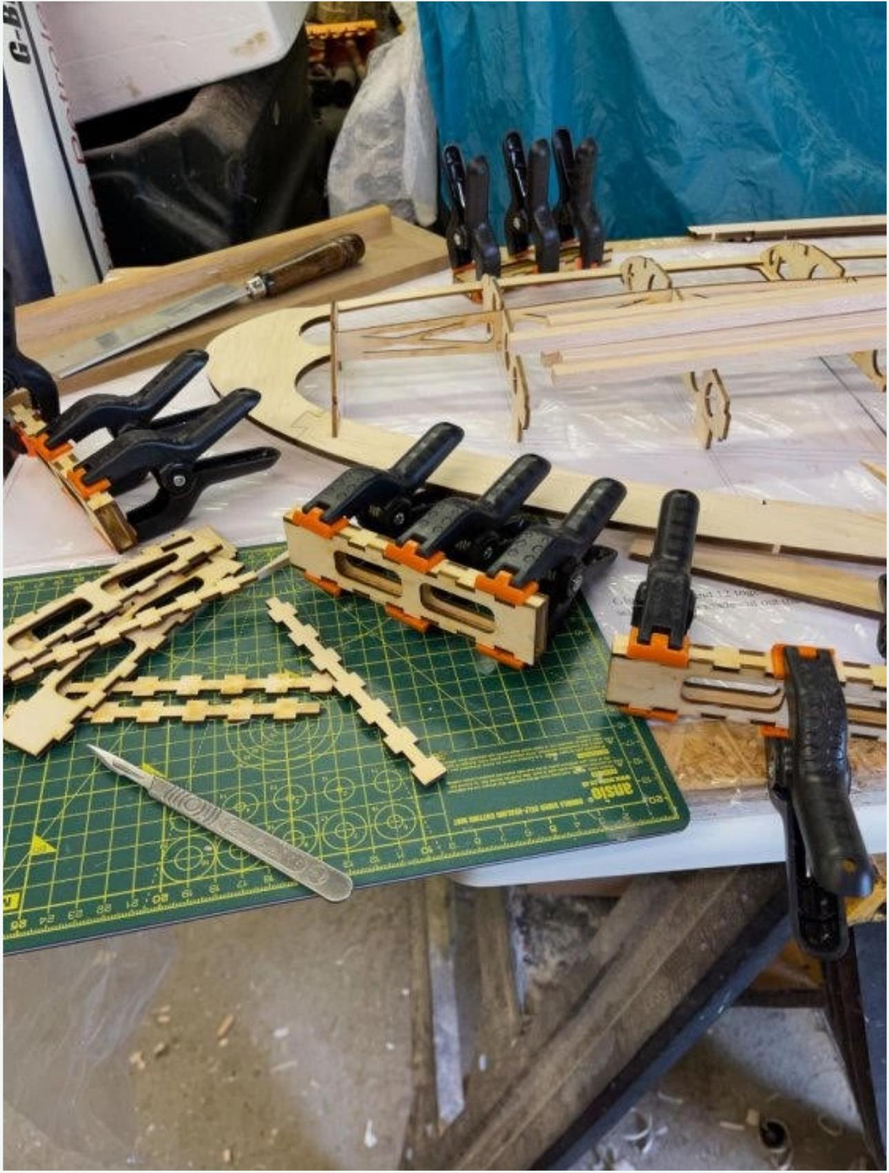
There was a lot of time spent waiting for glue to dry before I could move on to the next bit of the wing as I didn't want to build in a warp. The wing is free standing and rests on the rib tabs whilst the build takes place.
