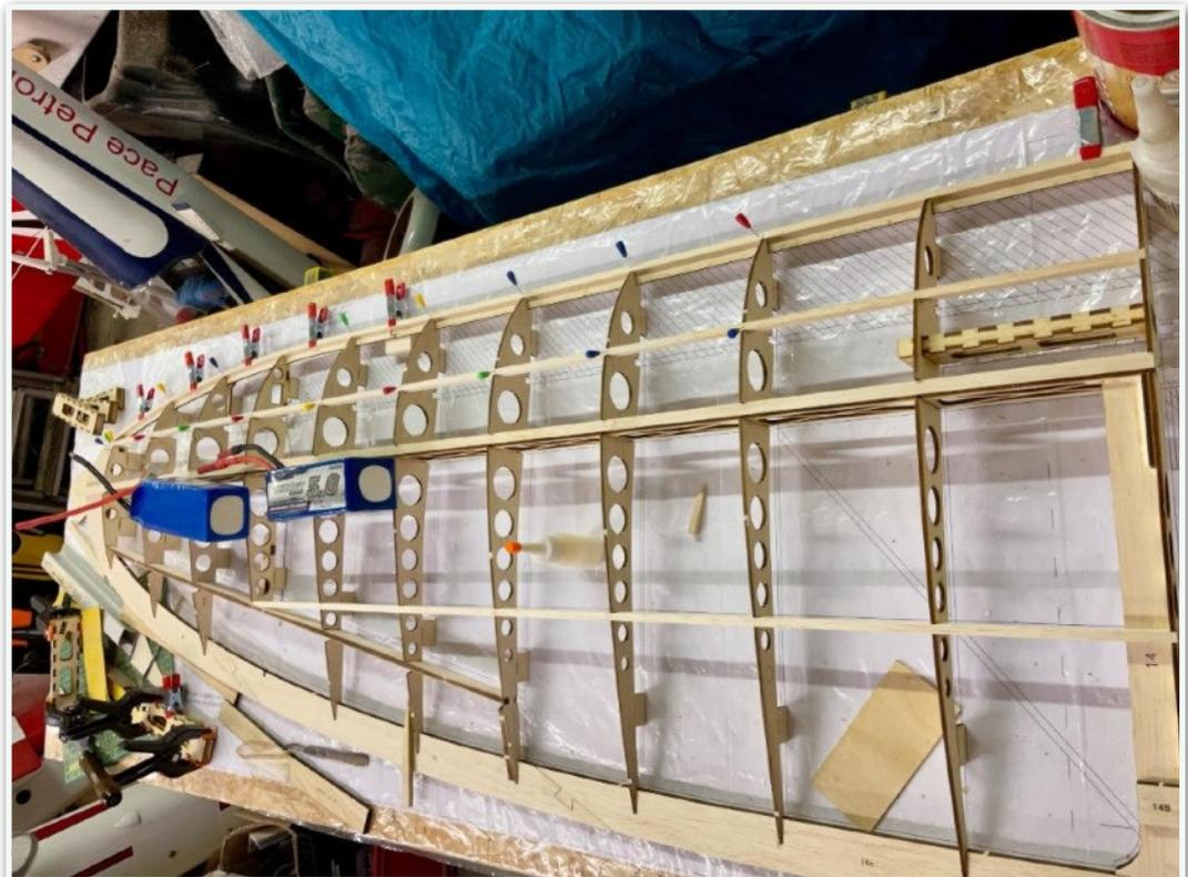
When dry the wing was turned over and the lower wing spars fitted together with LE strips (5mm x 5mm for sheet support) and when they were dry I was able to plane back for the LE sheeting.
