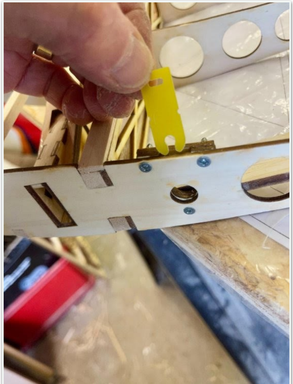
The clip slides in from the underside
