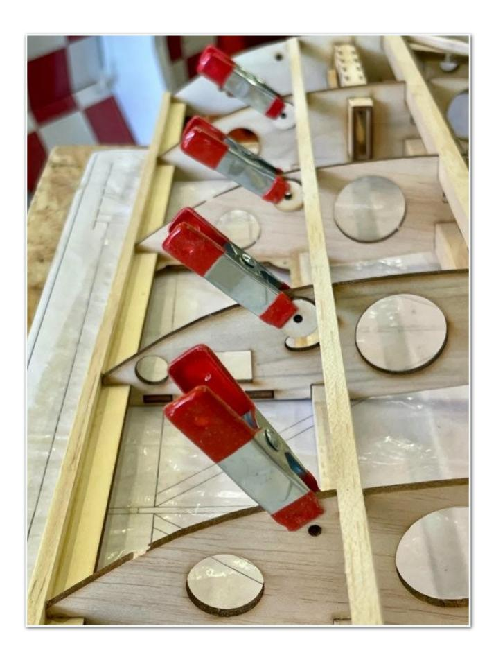
The air brakes with pivot levers attached.
