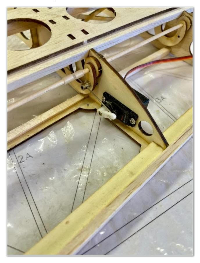
Having fitted the air brakes I then started to fit the balsa sheeting to the top of the wing but quickly realised that in doing so the air brakes wouldn't open. I needed to cut an internal chamfer on the LE of the air brakes so that they clear the balsa sheet, I should have looked more closely at the plan as it quite clearly shows said chamfer.
