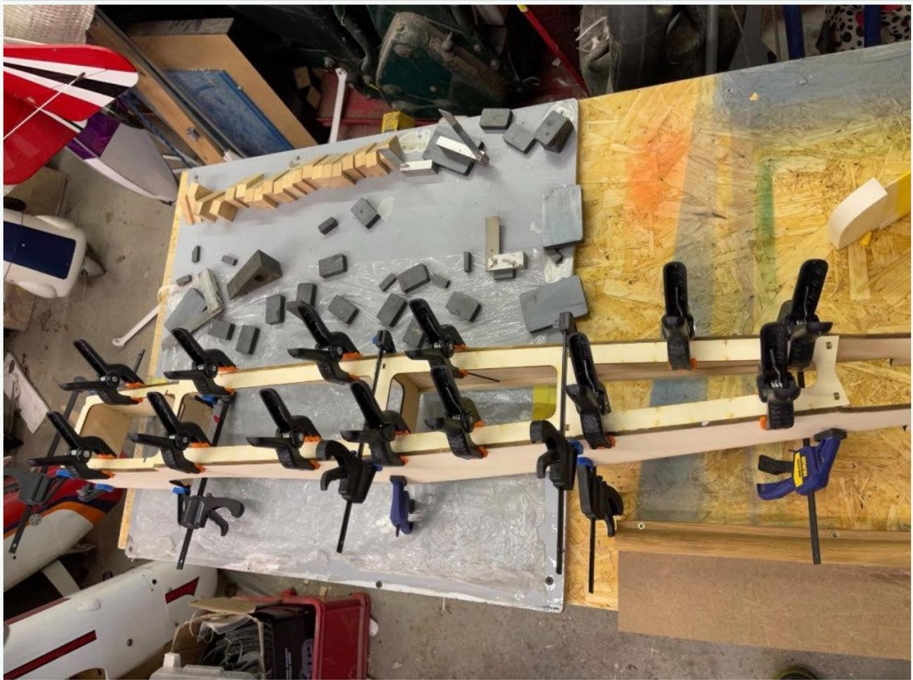
Whilst various bits were drying I started to look at the work needed to accommodate the SC 52s. The first is to move the firewall back, the shot below shows where it will have to sit to keep the nose in the same position
