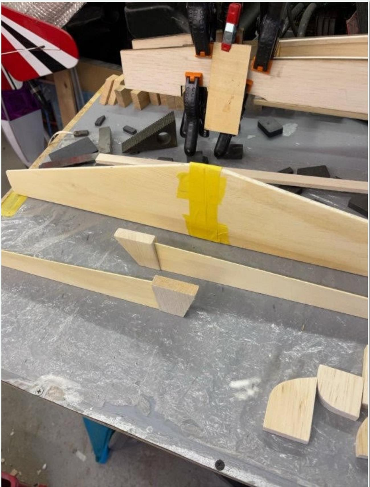
And these are the tip ends which will need to be cut and reformed due to my mistake in building the wrong model.
