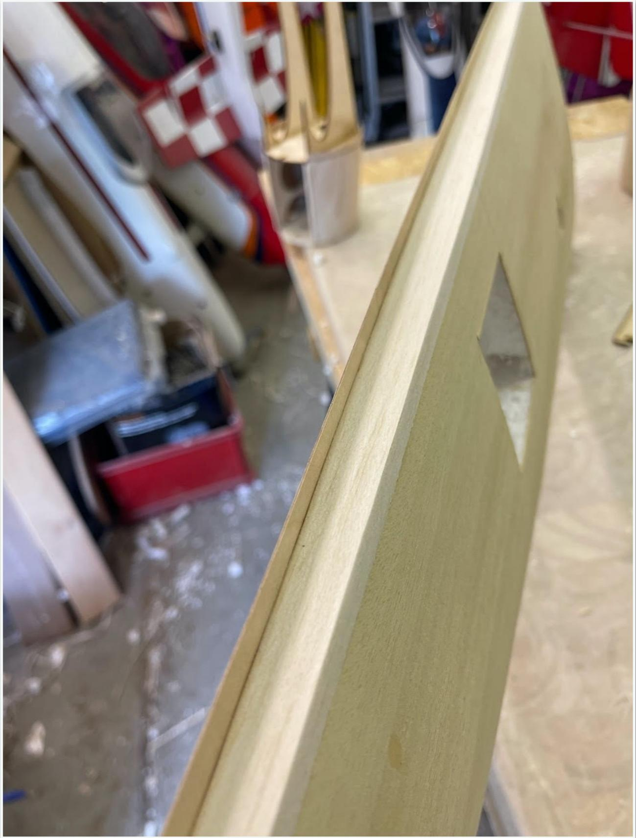
The 2 halves of the wing were then glued together (Gorilla Glue Brown).
