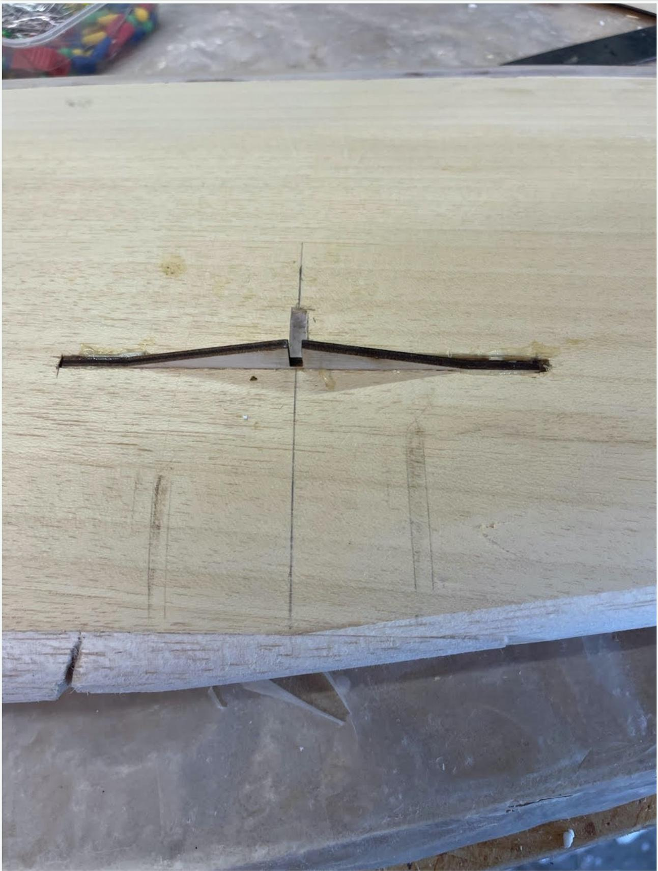
Other work carried out to the wing halves before joining them together was the fitting of the wingtips and the attachment of a thin strip of thin ply which will cover the aileron and flap hinge line. This is exactly the same as I did on my BF-110 which entailed sanding the top of the false TE to accommodate the thin ply.
