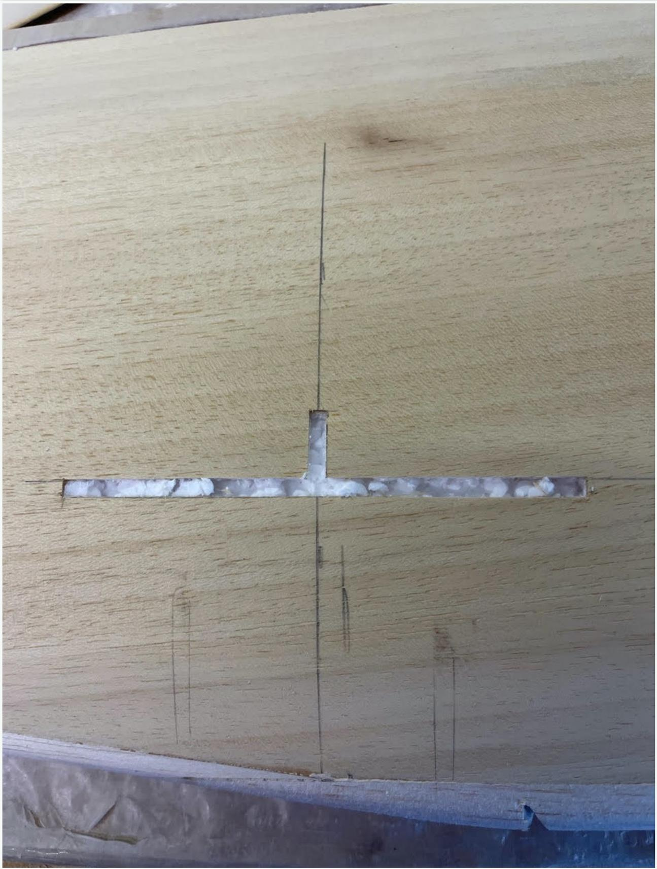
Then formed the slot using my converted soldering iron gun.
