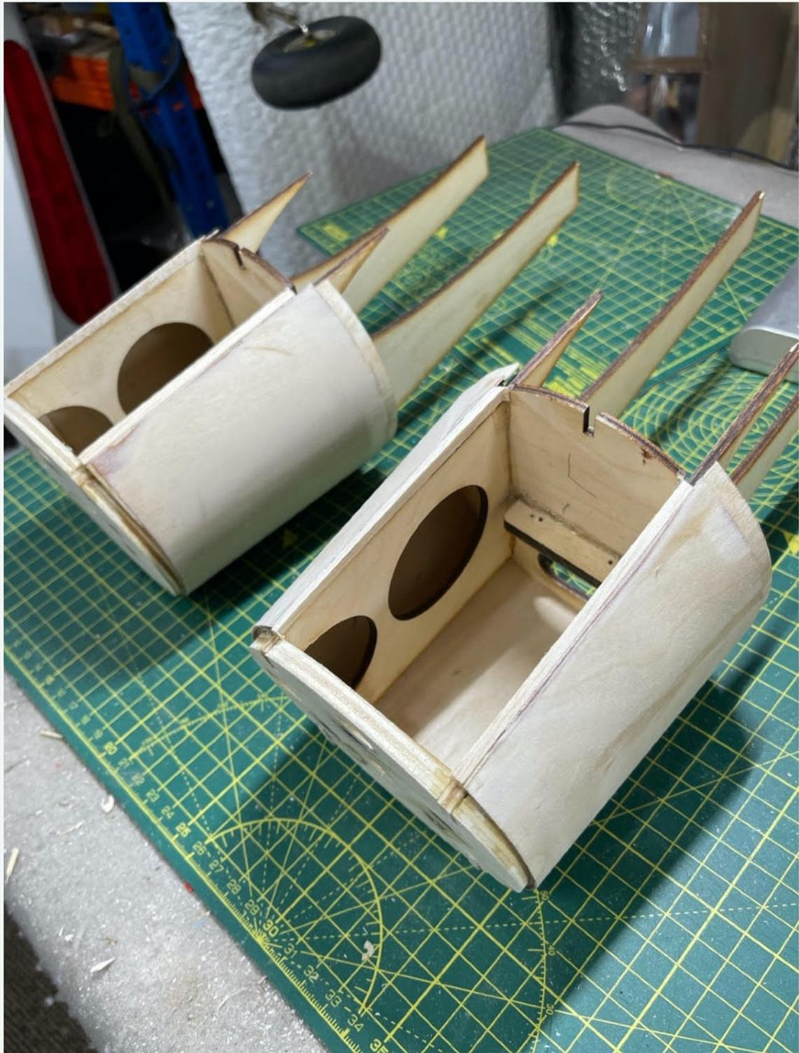
Checking the fit of the drainpipe engine cowling.
