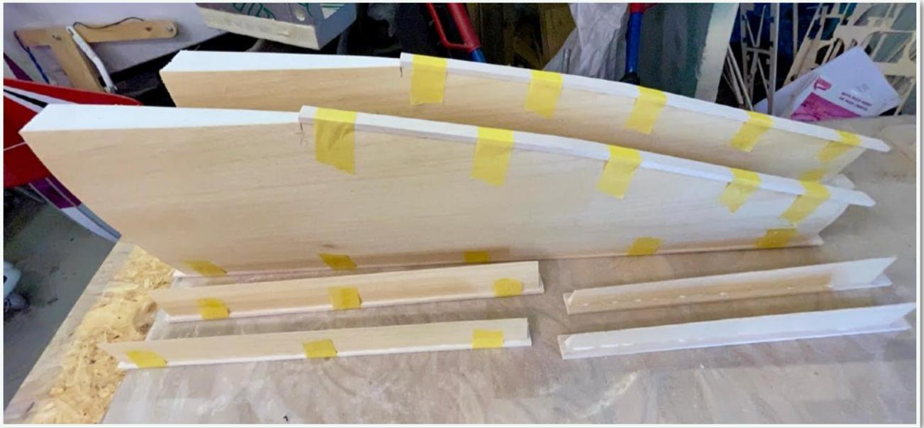
When the engine nacelles are attached to the wings they interlock with reinforcing plates which are sunk into the wings. So first I measured and marked their position in the top of the wing.
