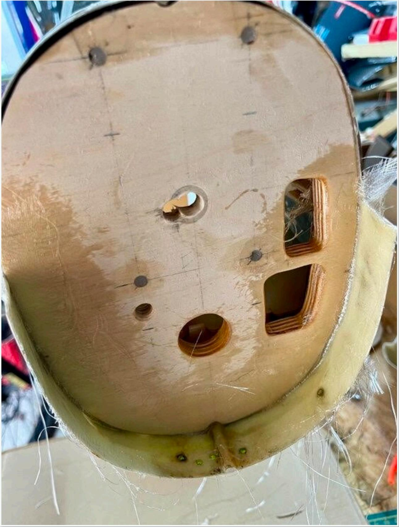
As with most IC, the height of the fuel tank can be critical but it is especially so with Laser engines and as their carbs sit quite high (low when inverted) the tank needs to go quite a bit lower than 'normal'. In order to achieve this a tank recess had to be cut in the top of the wing and the opening lined and glassed to maintain wing strength.
