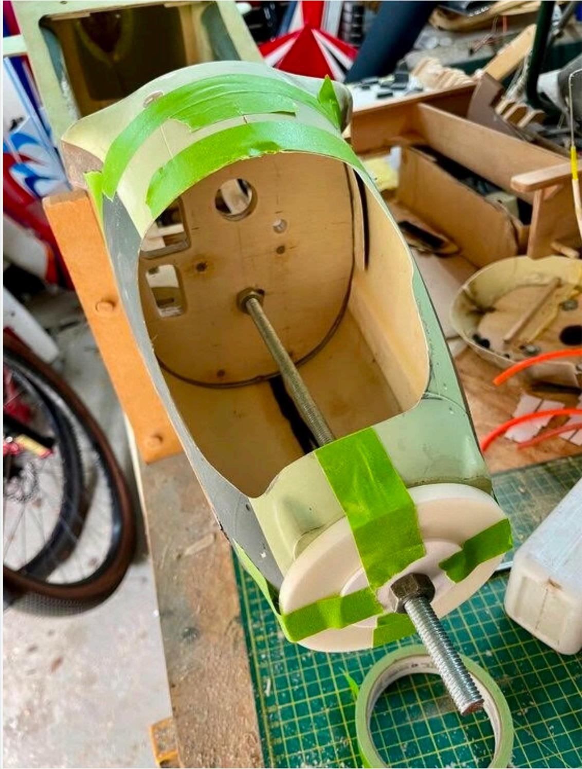
Once that had set I was then able to glass the front lower half from the front and the top upper half from the back. The large holes on the right are to allow the hot air to exit from the engine compartment.
