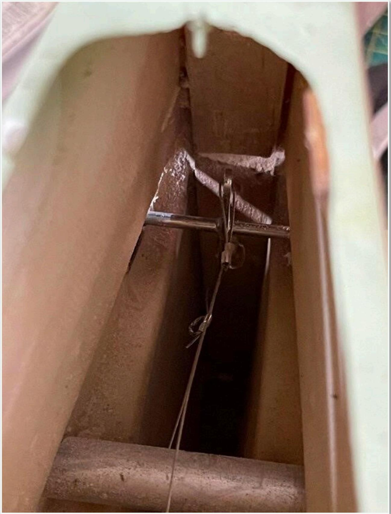
A new, raised servo tray had to be installed and the servos, together with pull pull for both rudder and elevators fitted.
