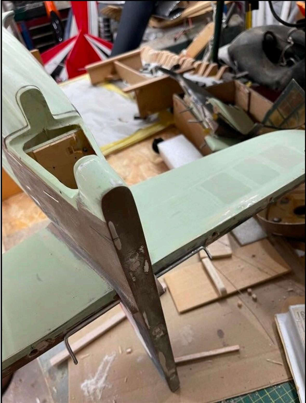
New elevator joiner with silver soldered control horn.
