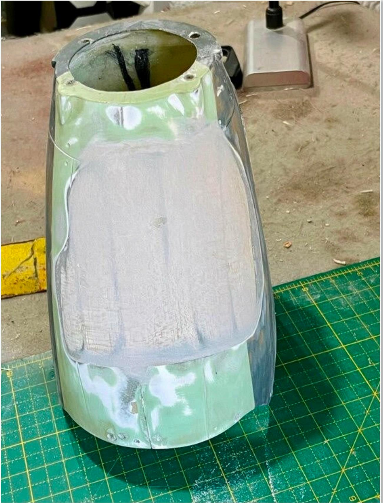
Holes cut for front pot and needle but you can see why I want to convert it to the tropical variant as the Vokes filter will not only cover the front pot but it will give me chance to sort some cool air ducting for the rear pot.
