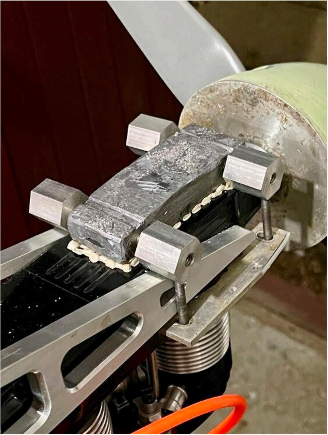
After machining it looks a bit better plus with the through bolts it gives me scope to have differing balance weights to put in place if I find this one to be less than ideal..
