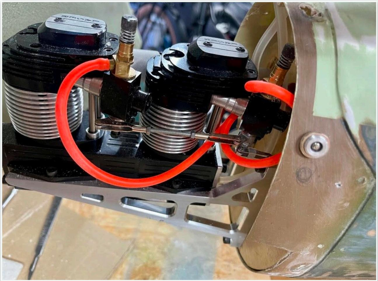
Couldn't resist putting it all together! I took the opportunity to use my Vanessa balancing rig the result being that I needed 500g of lead in the nose to get the correct C of G! This was initially zip tied to the motor.
