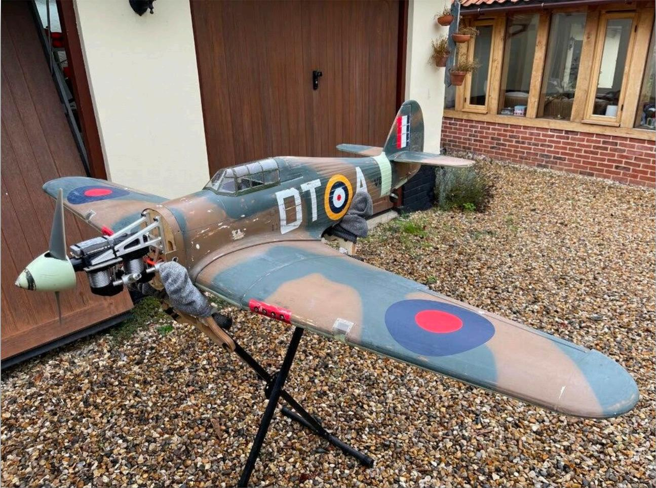
A few people thought that the zip tie arrangement to hold the lead in place might be tempting fate, so I changed it to a more positive fixing. This was the initial fabrication and I still needed to turn the hex bar down to make to look a bit less Frankenstein.
