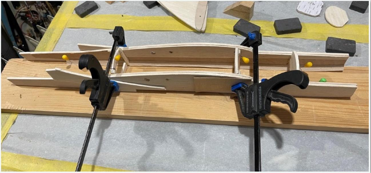
The build instructions and plans show a ply and balsa motor mount / rear former made by bending strips of ply around a former.
