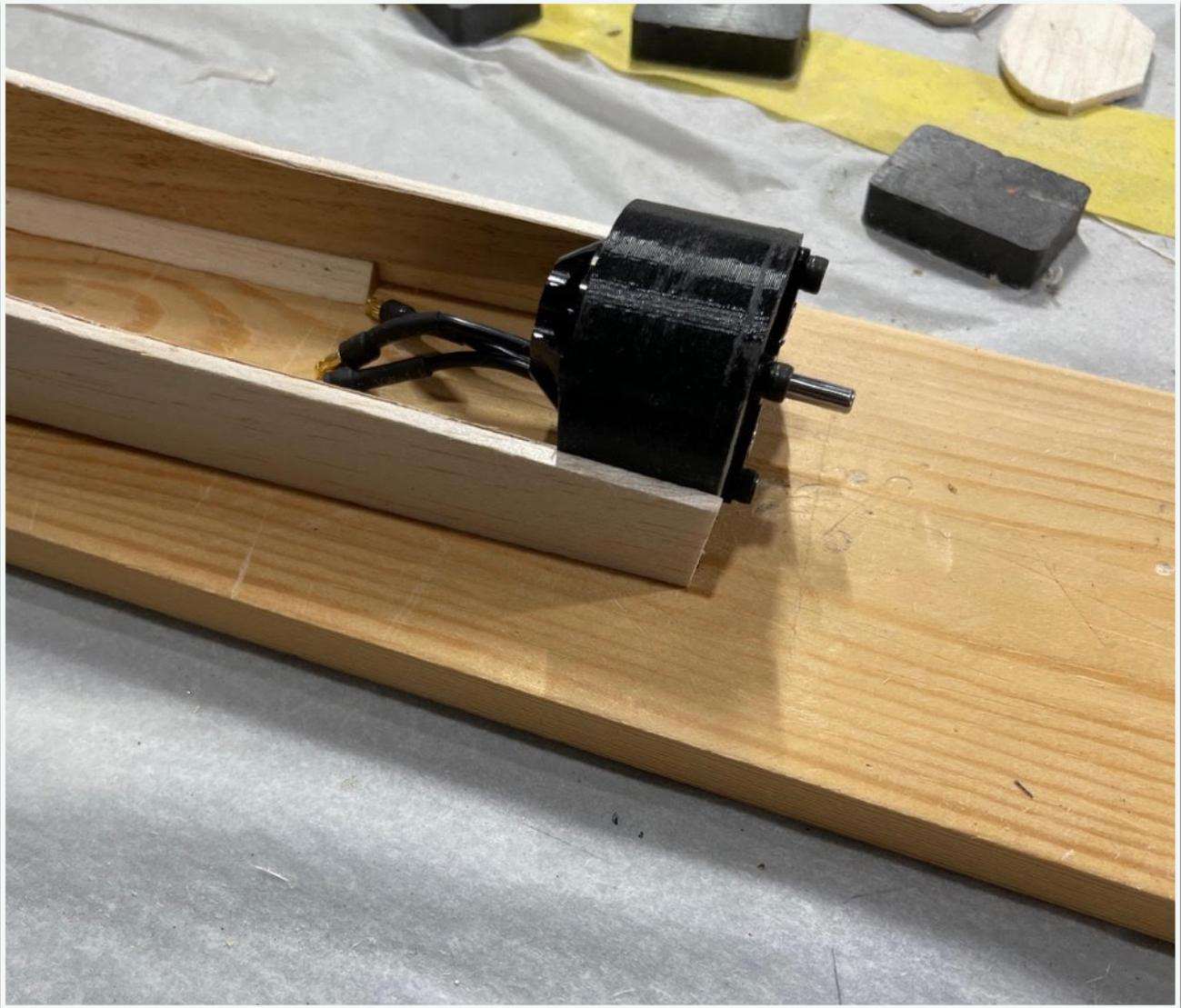
The front former was added as were the ply canopy side rails but they were held in place with double sided tape, the idea is the the canopy planking is stuck in place onto the ply side rails then it is cut out once dry
